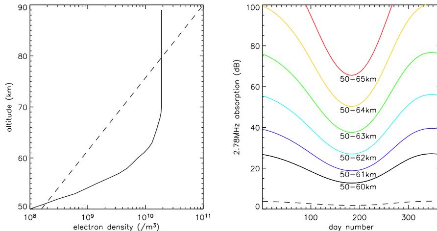
**Fig. 6.** Left: electron density profiles taken from Lübken et al. (2006) and presented as typical quiet (dashed line) and solar proton event disturbed (solid line). Right resulting integrated non-deviative absorption as a function of season. Computations for progressively higher upper limits for the integral (Eq. 1) are shown, and with the 50–60 km interval for the quiet situation shown as a dashed line.
