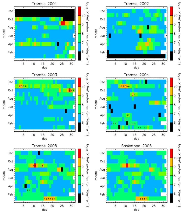
**Fig. 3.** Yearly tables of month vs. day for Tromsø the period 2001-5 inclusive. For days when ILME were detected (by our criteria) the total number of hours are indicated. The background colours indicate >1 MeV proton fluxes. Black indicates whenever the Tromsø MFR experienced operation problems of some kind. The lowest right-hand panel shows the corresponding statistics for Saskatoon 2005.
