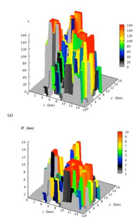
**Fig. 3.** A realization of cloud stochastic model that has a given power-spectral exponent, mean, and standard deviation. (a) optical depth filed; (b) cloud top height field.
