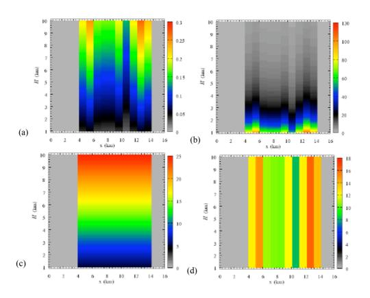
**Fig. 4.** An example of cloud microphysics. (a) liquid water content, LWC; (b) number of drops, N; (c) droplet effective radius,  $r_e$ ; (d) extinction coefficient,  $\sigma_{\rm ext}$ .
