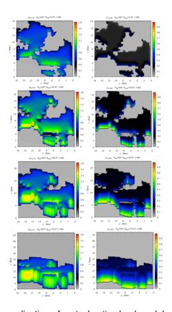
**Fig. 5.** Reflectance from a realization of a stochastic cloud model with constant cloud optical  $(\tau=80)$  and geometrical thicknesses (h=4 km). Left column:  $0.67 \,\mu\text{m}$ ; right column:  $2.1 \,\mu\text{m}$ ;  $\theta_0=60^\circ$ ;  $\theta=0^\circ$ ,  $20^\circ$ ,  $45^\circ$ , and  $70^\circ$ , from top to bottom. Note different color scales for left and right columns.
