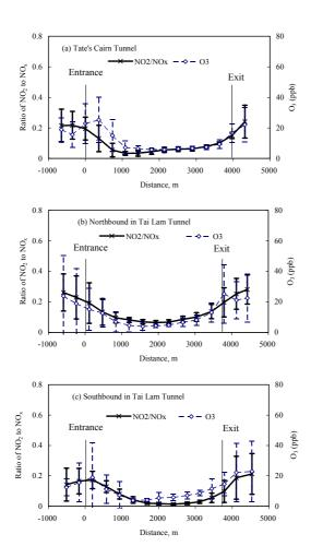
**Fig. 2.** Profiles of  $NO_2/NO_x$  and  $O_3$  in tunnels.
