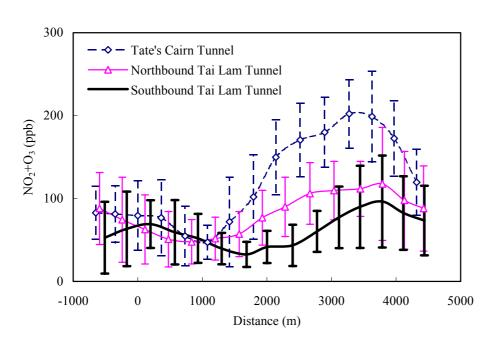
**Fig. 3.**  $(NO_2 + O_3)$  profiles in tunnels.
