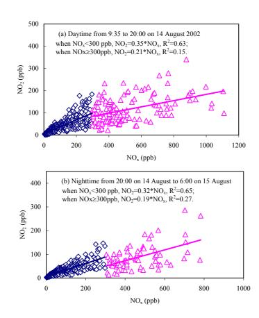
Fig. 5. Correlations between  $NO_2$  and  $NO_x$  in daytime and nighttime measurements.
