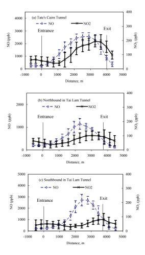
**Fig. 1.** Profiles of NO and NO<sub>2</sub> in tunnels.
