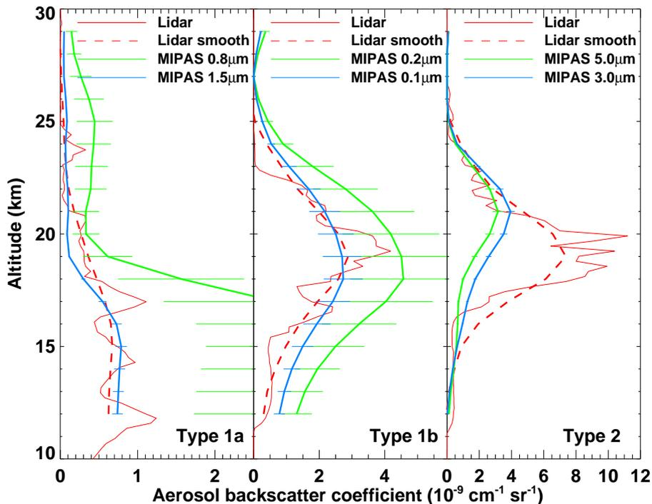
**Fig. 8.** Comparison of aerosol backscatter coefficients at 532 nm between Lidar measurements (red) and calculations based on MIPAS retrievals for two different median radii (green and blue). Solid red lines are the original lidar observations, while dashed ones are convolved with the averaging kernel of the MIPAS results. Error bars indicate the variation of the results for the range of refractive indices for NAT (Type 1a), STS (Type 1b), and ice (Type 2) from literature.
