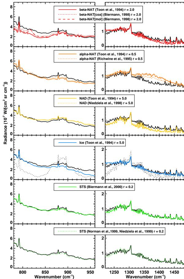
**Fig. 5.** Same plot as Fig. 4 but for MIPAS spectra on 14 June 2003 for a tangent altitude of 17.3 km (black) in comparison with radiative transfer simulations for different refractive indices (color) and a nearby PSC-free measurement (black, dotted). This observation occurred close to a Lidar measurement of Type 1b PSCs.
