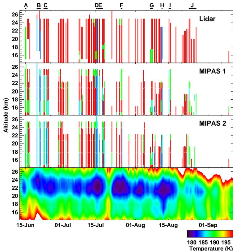
**Fig. 10.** Comparison between lidar and MIPAS PSC type analysis. For lidar, red indicates Type 1a, green Type 1b and blue Type 2 PSC. In case of MIPAS red stands for R1, blue for R2, green for R3, and blue-green for region R4 in Fig. 9. “MIPAS 1” indicate the nearest and “MIPAS 2” the second nearest MIPAS limb-scan with respect to the lidar observation in terms of  $\Delta t_{\text{of}}$  (see text). A–J denote periods discussed in the text.
