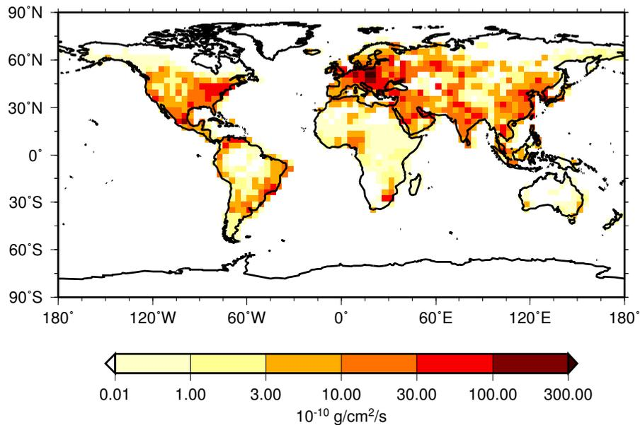
**Fig. 1.** NO<sub>x</sub> emission [ $10^{-11} \text{ gcm}^{-2} \text{ s}^{-1}$ ] from road traffic in 1990.
