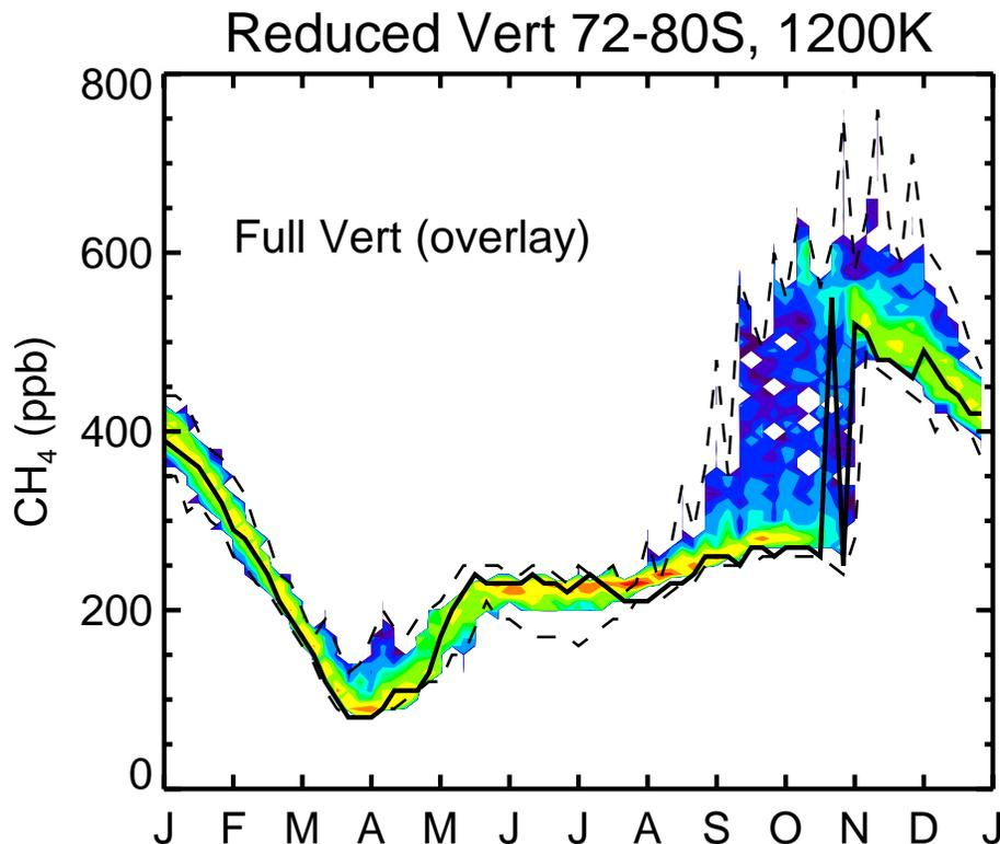
**Fig. 7.** The annual cycle of model CH<sub>4</sub> 72–80° S on the 1200 K surface using contoured pdfs. Yellow and red are high values of the most probable mixing ratio, and purple and blue indicate low probability, or infrequently observed mixing ratios. Reduced Vert is shown in color and the outline of the mean (solid) and range (dashed) for Full Vert is overlaid.
