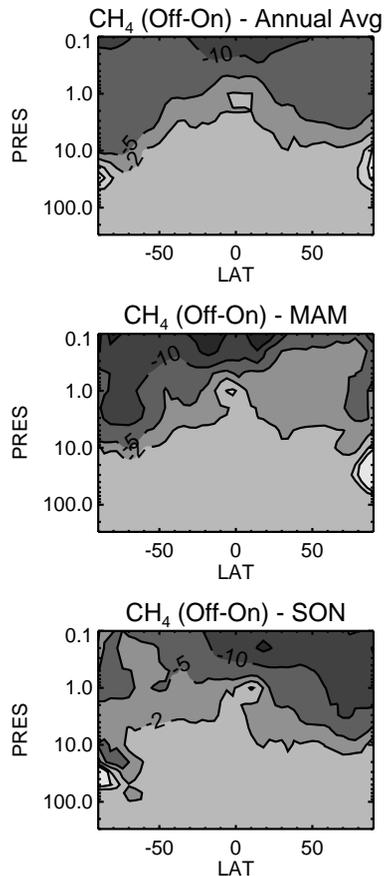
**Fig. 3.** Percentage difference in CH<sub>4</sub> distributions between the offline CTM calculation and an online chemical calculation in a GCM ( $(\text{offline-online})/\text{online} \times 100\%$ ). Top to bottom: annual average, March-April-May mean, and September-October-November mean. The vertical coordinate is pressure (hPa).
