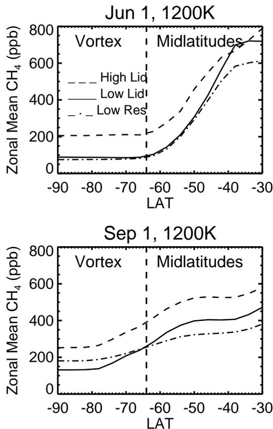
**Fig. 15.** Methane meridional gradients in the SH for High Lid (dashed), Low Lid (solid), and Low Res (dot-dash). The gradients of the three simulations are similar in late fall (top), but by the end of winter (bottom), the Low Res gradient between the midlatitudes and the vortex is much flatter than the two  $2^\circ \times 2.5^\circ$  simulations.
