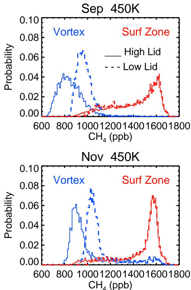
**Fig. 12.** Comparison of the separation of vortex (60–80° S, blue) and midlatitude (44–60° S, red) air masses in High Lid (solid) and Low Lid (dashed) in September and November. The lid height does not affect the midlatitude distributions, but the High Lid vortex maintains lower CH<sub>4</sub>.
