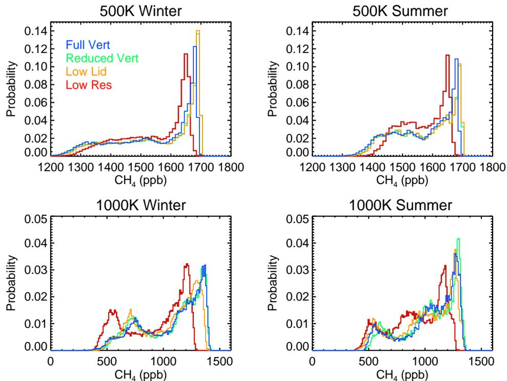
**Fig. 6.** Probability distribution functions (pdfs) of CH<sub>4</sub> at 500 K (top panels) and 1000 K (bottom panels) in winter (left) and summer (right) for 4 CTM simulations. Full Vert (blue), Reduced Vert (green), and Low Lid (orange) all have 2°×2.5° resolution and nearly the same tropical-midlatitude separation. Low Res (red) produces a subtropical mixing barrier, but peak separation differs from the higher resolution models.
