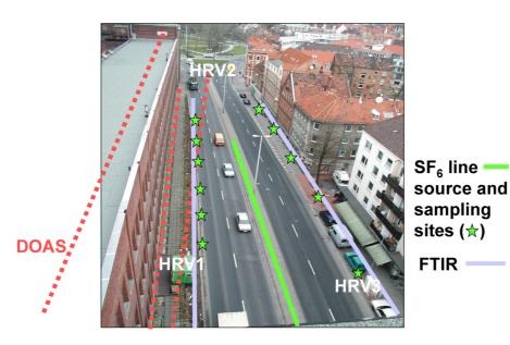
**Fig. 1.** Street Canyon "Goettinger Strasse" with instrumentation. The picture shows the continuous monitoring stations HRV1 to HRV3 in white and the SF6-line-source at the median strip plus the sampling bag locations in green colour. The path-averaged measurements are indicated by the blue (FTIR) and red (DOAS) lines.
