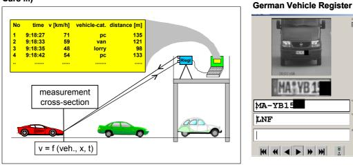
Fig. 3. Experimental set-up for traffic counts and vehicle speed measurements.
