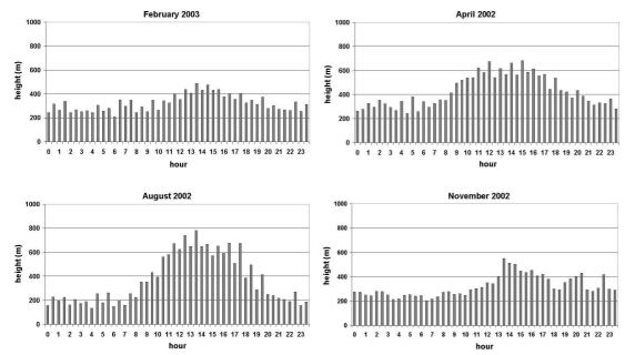
Fig. 5. Monthly mean mixing-layer height over the city of Hanover (Germany) derived from SODAR measurements for four months from the four seasons (from Emeis and Türk, 2004).
