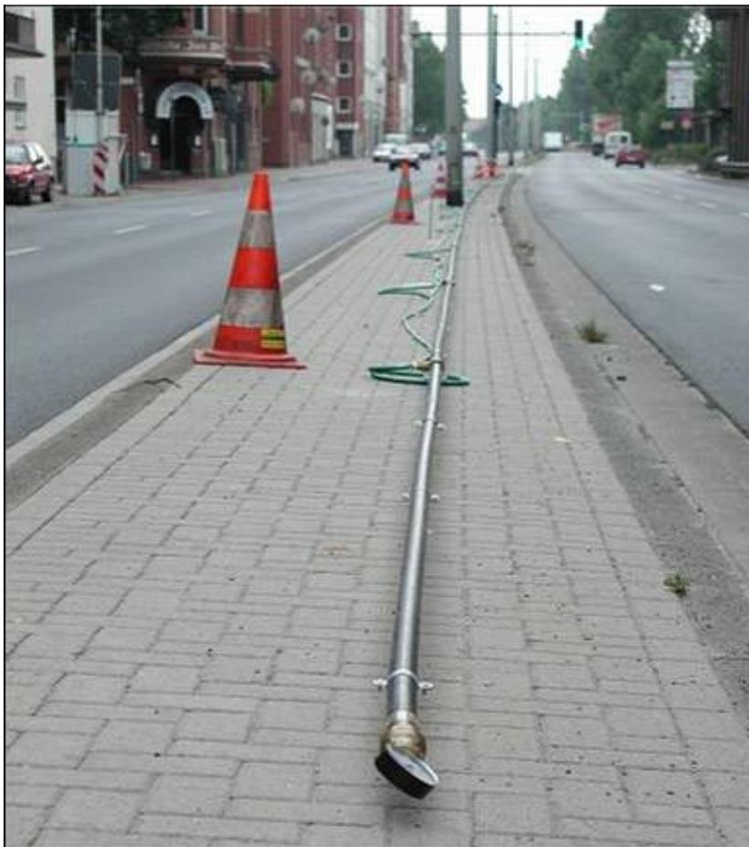
**Fig. 2.** Picture of the 96 m long SF<sub>6</sub> line source which was positioned on the median strip of the street canyon.
