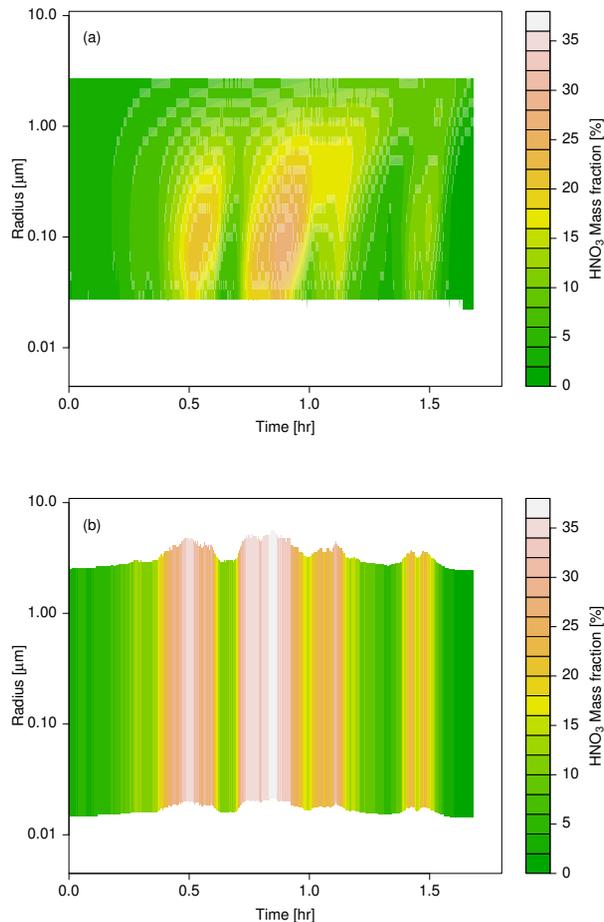
**Fig. 10.** The changes in HNO<sub>3</sub> mass fraction across the particle size range during the  $T_{\text{UCSE}} + 1.5 \text{ K}$  model run shown in Fig. 8 for **(a)** our microphysical model and **(b)** the equilibrium model.
