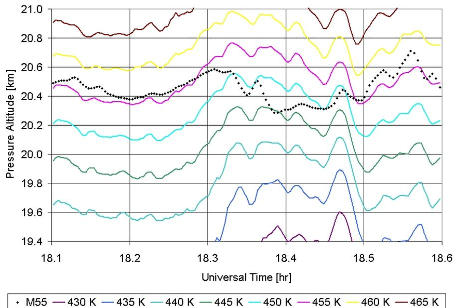
**Fig. 5.** Comparison of the pressure altitude of the Geophysica-M55 during the flight on the 8 February 2003 (black diamonds) with the pressure altitudes of isentropic surfaces (coloured solid lines) at 5 K intervals.
