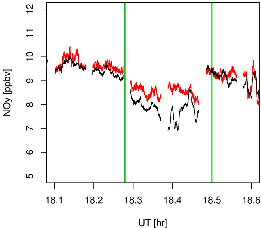
**Fig. 3.** Measured total (gas-phase plus  $3.6 \times$  particle-phase; red line) and gas-phase (black line)  $\text{NO}_y$  measured by the SIOUX instrument around the second PSC event on the flight on 8 February 2003. The green lines denote the edges of the region of PSCs marked by the green line in Fig. 2.
