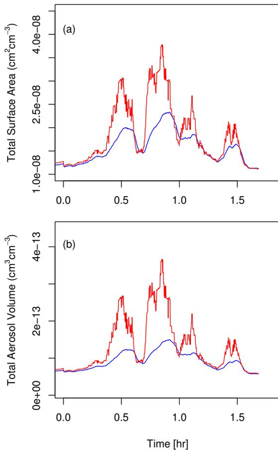
**Fig. 11.** Comparisons of the total aerosol **(a)** surface area and **(b)** volume produced from the equilibrium (red lines) and dynamic (blue lines) models in the  $T_{UCSE} + 1.5\text{ K}$  test case.
