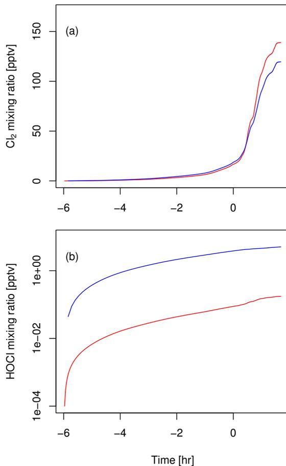
**Fig. 12.** Production of **(a)** Cl<sub>2</sub> and **(b)** HOCl during the T<sub>UCSE</sub> + 1.5 K model runs shown in Fig. 8. The blue line indicates the output from our microphysical model, the red line that from the equilibrium code.
