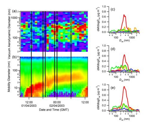
**Fig. 7.** The 1 April growth event as observed by the AMS **(a)** and DMPS **(b)**. Distributions **(c)**, **(d)** and **(e)** are from 13:00–18:00, 19:00–23:00 and 00:00–06:00 GMT respectively. Note that the composition is partly inorganic during the later stages.
