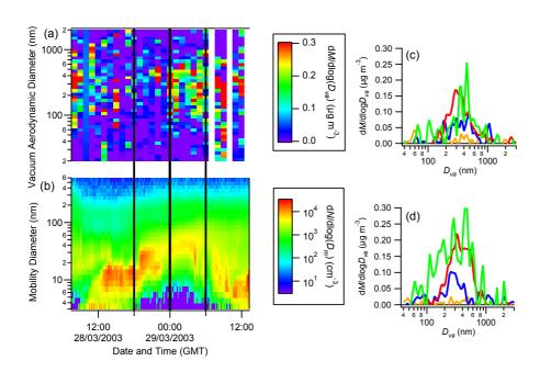
**Fig. 6.** The 28 March nucleation and growth event. **(a)** is the AMS-measured organic mass distribution, while **(b)** is the DMPS-measured number concentrations. **(c)** is the AMS distribution from 18:00 to 00:00 GMT, while **(d)** is from 00:00 to 06:00 the following day. These periods are indicated by the black lines on (a) and (b) for convenience.
