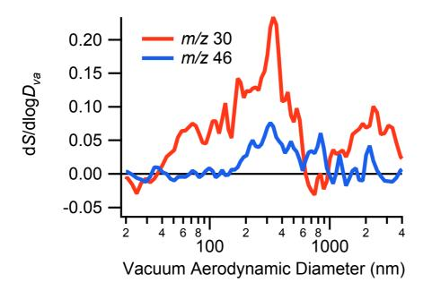
**Fig. 9.** Graph comparing the m/z 30 and 46 signals from the period of 00:00 to 06:00 GMT on 2 April, during the later stages of a growth event. The accumulation mode (150–600 nm) signal ratios is typical of ammonium nitrate, while the coarse mode (>1  $\mu$ m) is probably sodium nitrate. However, the Aitken mode (<150 nm) is something else, potentially an organic nitrogen species.
