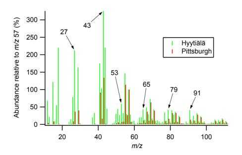
**Fig. 8.** Comparison between the organic mass spectral signatures of a growth event at Hyytiälä and primary traffic emissions extracted from ambient sampling in Pittsburgh (Zhang et al., 2005). The spectra are presented relative to m/z 57, the largest aliphatic peak that does not receive significant contributions from other sources.
