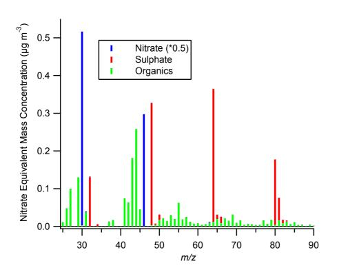
**Fig. 4.** Mass spectral signature for nitrate, sulphate and organics during the continental outbreak. The nitrate values have been halved for clarity. This pattern is typical of regional pollution observed using the AMS.
