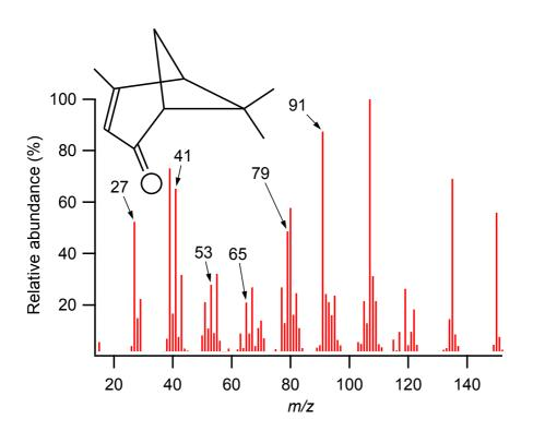
**Fig. 10.** Molecular structure and mass spectrum of verbenone, taken from the NIST database (2003). Some the unexpected peaks present in the ambient data are labelled. m/z 39 is not present in the AMS data shown previously, as it is routinely rejected due to interferences from thermally-ionised potassium. The listed higher mass fragments are also not present, but these are almost certainly lost through thermal decomposition during flash vaporisation.
