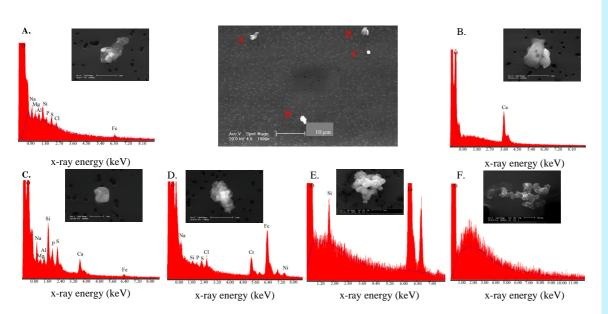
**Fig. 3.** Secondary electron images and EDX spectra of residual ice crystals collected during INTACC. Inserts **A.**, **B.**, **C.**, and **D.**, are detailed micrographs of the larger micrograph shown in the upper row, middle column. Inserts **E.** and **F.** do not appear in the larger micrograph.
