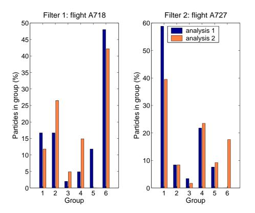
**Fig. 1.** Percentage of particles falling into each category for the two duplicate samples analyzed on Flight A718 (filter 01) and on Flight A727 (filter 02). The abundance of the elements in each group is shown in more detail in Table 3 (for analyses 1).
