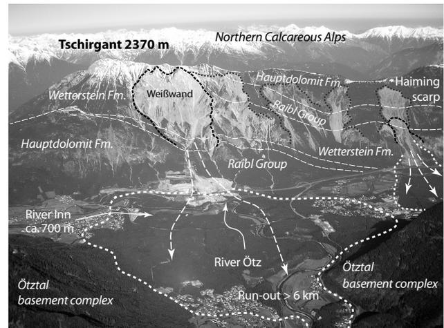
**Fig. 3.** Oblique view to the northern Ötz- and Inn-valley: scarp (black stippled) and accumulation areas (white stippled) of the Tschirgant and Haiming rockslides (photo courtesy of M. Schuster 2007).
