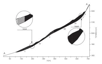
**Fig. 5.** Cross section A-A', splitting the slope into rock blocks (location – see Fig. 3). Roman numbers indicate the granulometric classes defined during field investigations and summarized in Table 1.
