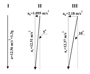
Fig. 6. Considered cases of seismic acceleration.
