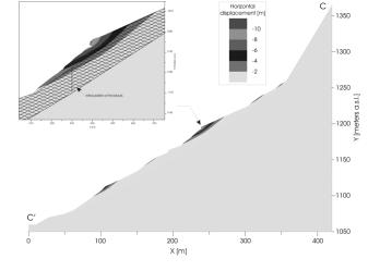
**Fig. 7.** Field of horizontal displacement in C-C' cross-section (location – see Fig. 3). Acceleration case II.
