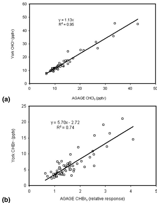
**Fig. 1.** (a) Organic correlation of York and Bristol CHCl<sub>3</sub> mixing ratios measured during the NAMBLEX campaign, using data points taken within the same 40-min period. (b) Organic correlation of York CHBr<sub>3</sub> mixing ratios and Bristol CHBr<sub>3</sub> relative response data, using data points taken within same 40-min period.
