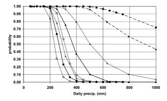
**Fig. 15.** Exceedance probabilities in 50 years. Squares, raw-data; triangles,  $\log_{10}$ -data. Thick lines-filled markers, median of posterior distribution; thin lines-hollow markers, 0.05 and 0.95 quantiles. Probability of attainable precipitation, dashed lines.
