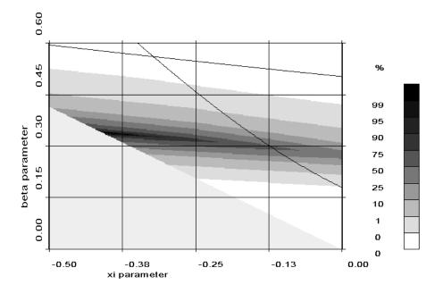
**Fig. 8.** Significance of KS goodness-of-fit test,  $\alpha(\xi, \beta)$ , for log<sub>10</sub>-data. u=1.653 mm.
