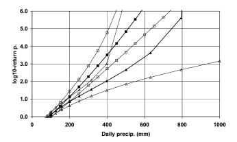
**Fig. 14.** Estimated  $\log_{10}$ -return periods,  $\log_{10} \tau(x)$ . Squares, raw-data; triangles,  $\log_{10}$ -data. Thick lines-filled markers, median of posterior distribution; thin lines-hollow markers, 0.05 and 0.95 quantiles.
