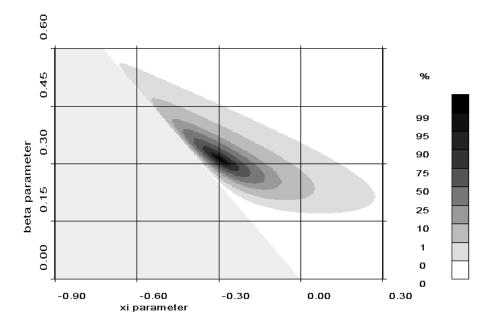
**Fig. 3.** Posterior density of  $\xi$ ,  $\beta$  for  $\log_{10}$ -data.  $u = 1.653 = \log_{10}(45)$ . Flat prior. High probability of Weibull DA. Lower-left grey triangle is a null-likelihood zone due to observations.
