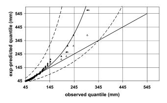
**Fig. 5.** QQ-plot with GPD( $\xi$ =0) as reference (diagonal line). Sample distribution of log<sub>10</sub>-data: filled and hollow markers correspond to upper and lower corners of the stepwise function; maximum like-lihood estimated GPD, full line; dotted lines: 5% acceptance region for Kolmogorov-Smirnov test.
