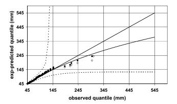
**Fig. 4.** QQ-plot with GPD( $\xi$ =0) as reference (diagonal line). Sample distribution of raw-data: filled and hollow markers correspond to upper and lower corners of the stepwise function; maximum like-lihood estimated GPD, full line; dotted lines: 5% acceptance region for Kolmogorov-Smirnov test.
