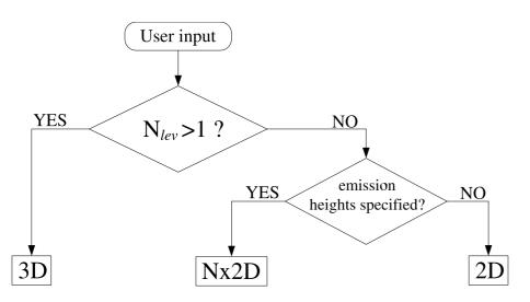
**Fig. 1.** OFFLEM flowchart: Logic for the determination of the emission *type*: if the vertical dimension ( $N_{lev}$ ) of the user defined input field is larger than 1, the emission *type* is 3-D, if the vertical dimension is 1, the presence of the z-specifier is the marker to distinguish between Nx2D (emission height specified) and 2-D emission *type*. (Note: The vertical dimension ( $N_{lev}$ ) of a Nx2D field is 1, whereas its invariant parameter dimension ( $N_{par}$ ) equals N.)
