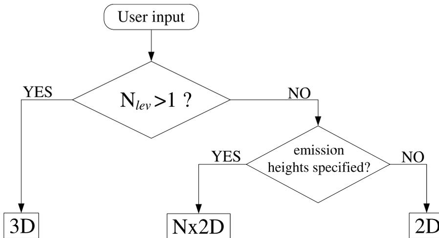
**Fig. 1.** OFFLEM flowchart: Logic for the determination of the emission *type*: if the vertical dimension ( $N_{lev}$ ) of the user defined input field is larger than 1, the emission *type* is 3-D, if the vertical dimension is 1, the presence of the z-specifier is the marker to distinguish between Nx2D (emission height specified) and 2-D emission *type*. (Note: The vertical dimension ( $N_{lev}$ ) of a Nx2D field is 1, whereas its invariant parameter dimension ( $N_{par}$ ) equals N.)
