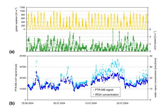
**Fig. 3. (a)** Time series of global radiation and wind speed for the study period; **(b)** time series of water vapour concentration as measured by the open-path IRGA and the normalised m37 signal detected by PTR-MS.
