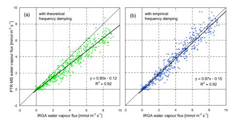
**Fig. 6.** Comparison of water vapour fluxes obtained with PTR-MS and open-path IRGA. Only quality checked IRGA data (n=450). (a) PTR-MS flux with theoretical high-frequency correction after Moore (1986); (b) PTR-MS flux with empirical high-frequency correction.
