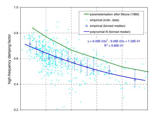
**Fig. 5.** Empirically determined high-frequency damping factors plotted against wind-speed. The 2nd order polynomial fit to the median values of wind speed classes are displayed as solid curve and numerical function. For comparison, the damping factor by the spectral transfer parameterisation after Moore (1986) is also shown.
