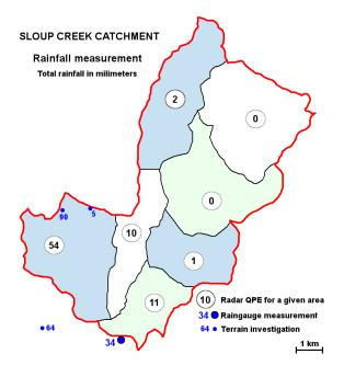
**Fig. 8.** Rainfall accumulation in Sloup creek catchment on 26 May 2003 from 12:00 to 16:00 CET. Areal radar-based QPE, rainfall measured by raingages and rainfall obtained by terrain investigation. The rainfall accumulation measured by radar was underestimated roughly by factor of 0.9.
