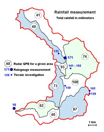
**Fig. 3.** Rainfall accumulation in Hodoninka river basin on 15 July 2002 from 15:00 to 21:00 CET. Areal adjusted radar-based QPE, rainfall measured by raingages and rainfall obtained by terrain investigation. The rainfall accumulation measured by radar was underestimated roughly by factor of 0.6.
