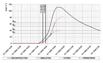
**Fig. 4.** Discharge forecasts at Štěpánov profile, 17:30 and 17:50 CET. The first warning of danger of flood could have been given 50 min, the second warning 30 min before large flooding in Štěpánov town. The villages situated at higher altitudes were already flooded.
