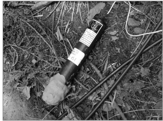
Fig. 4. No-polarizable electrode: Pb-PbCl 2 .
