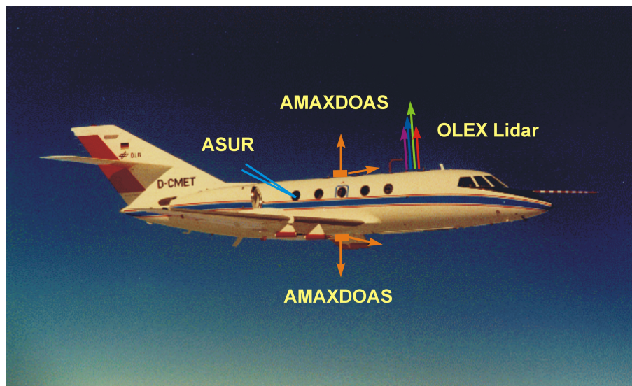
Fig. 2. The German Aerospace Center's meteorological research aircraft Falcon 20 equipped with the three remote sensing instruments ASUR, AMAXDOAS, and OLEX for airborne validation of SCIAMACHY data products O_3 , N_2O , NO_2 , BrO , H_2O , OCIO , and cloud and aerosol optical properties.
