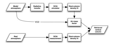
**Fig. 2.** Illustration of the empirical air-mass factor approach. High resolution spectra are generated with a radiative transfer model. A SCIAMACHY simulator converts this to spectra with the appropriate instrument resolution. Subsequently a DOAS fit is performed for the modelled spectrum and the air-mass factor is the ratio of the fitted slant column divided by the vertical column used in the radiative transfer calculation.
