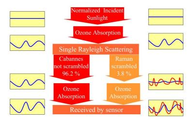
**Fig. 1.** Illustration of changes in the light intensity starting at the sun, crossing the atmosphere and moving to the satellite, for elastic (left part) and inelastic (right part) scattering. The blue lines represent the wavelength dependence of the ozone cross section, the red line represents the reflectance spectrum of inelastic scattered light.
