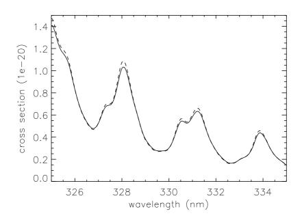
**Fig. 3.** A plot of the GOME Flight Model (dotted line) and SCIAMACHY Flight Model (solid line) cross sections for the 325-335 nm window. Both cross sections are broadened to the same spectral resolution as discussed in the text.
