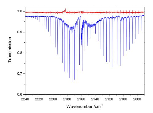
**Fig. 4.** FT-IR spectrum of the CD stretching region of a  $^{12}$ CH $_3$ Cl and CD $_3$ Cl mixture during reaction with Cl atoms. The  $\nu_1(A_1)$  and  $2\nu_5(A_1+E)$  modes of CD $_3$ Cl are overlapped by the sharp vibration-rotation lines of the CO fundamental centred at  $2043\,\text{cm}^{-1}$ . The topmost curve is the residual of the spectral fitting. Compounds included in the spectral analysis: CD $_3$ Cl, H $_2$ O, HDO, CO and CO $_2$ .
