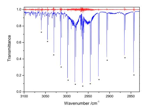
**Fig. 2.** FT-IR spectrum of the CH stretching region of a  $CH_3CI$  and  $^{13}CH_3CI$  mixture during reaction with CI atoms. Total photolysis time: 2 min. Compounds included in the spectral analysis:  $^{12}CH_3CI$ ,  $^{13}CH_3CI$ ,  $H_2O$  and HCI. (\*) Bands due to HCI.
