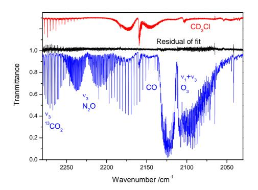
**Fig. 8.** FT-IR spectrum of the CD stretching region of a  $CH_3CI$  and  $CD_3CI$  mixture during reaction with OH radicals. The spectrum was analyzed in terms of  $CO_2$ , CO,  $N_2O$ ,  $H_2O$  and  $O_3$  reference spectra from the HITRAN database and of the shown high resolution reference spectrum of  $CD_3CI$ , which has been shifted for the sake of clarity.
