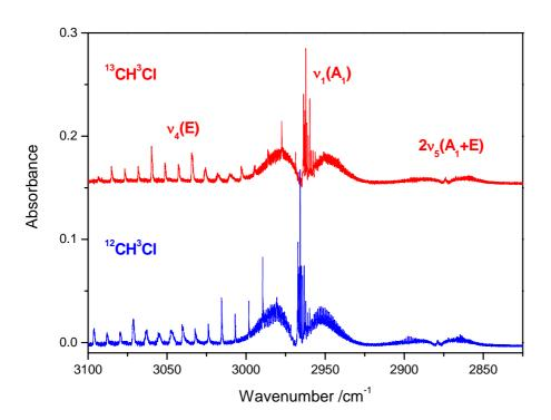
**Fig. 1.** FT-IR spectra in the CH stretching region of a CH<sub>3</sub>Cl and  $^{13}$ CH<sub>3</sub>Cl showing the fundamental  $\nu_1$  parallel band around 2960 cm<sup>-1</sup>, the  $\nu_4$  perpendicular band around 3040 cm<sup>-1</sup>, as well as the  $2\nu_5$  overtone around 2875 cm<sup>-1</sup>. Spectral resolution: 0.01 cm<sup>-1</sup>.
