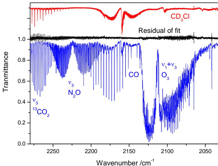
**Fig. 8.** FT-IR spectrum of the CD stretching region of a  $\text{CH}_3\text{Cl}$  and  $\text{CD}_3\text{Cl}$  mixture during reaction with OH radicals. The spectrum was analyzed in terms of  $\text{CO}_2$ , CO,  $\text{N}_2\text{O}$ ,  $\text{H}_2\text{O}$  and  $\text{O}_3$  reference spectra from the HITRAN database and of the shown high resolution reference spectrum of  $\text{CD}_3\text{Cl}$ , which has been shifted for the sake of clarity.
