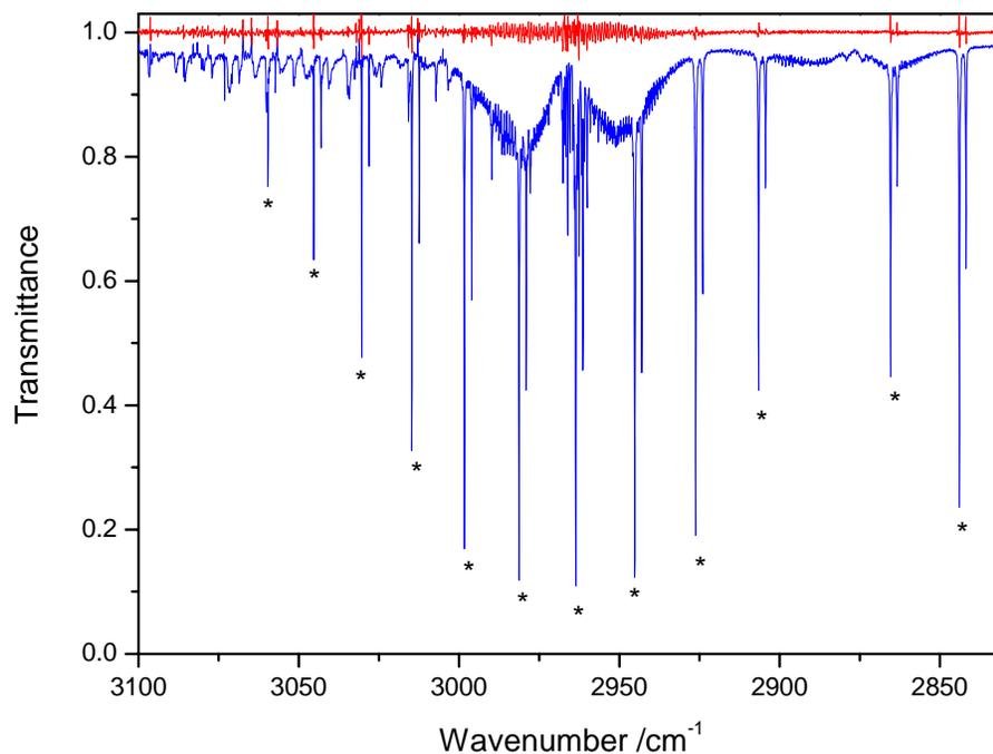
**Fig. 2.** FT-IR spectrum of the CH stretching region of a  $\text{CH}_3\text{Cl}$  and  $^{13}\text{CH}_3\text{Cl}$  mixture during reaction with Cl atoms. Total photolysis time: 2 min. Compounds included in the spectral analysis:  $^{12}\text{CH}_3\text{Cl}$ ,  $^{13}\text{CH}_3\text{Cl}$ ,  $\text{H}_2\text{O}$  and  $\text{HCl}$ . (\*) Bands due to  $\text{HCl}$ .
