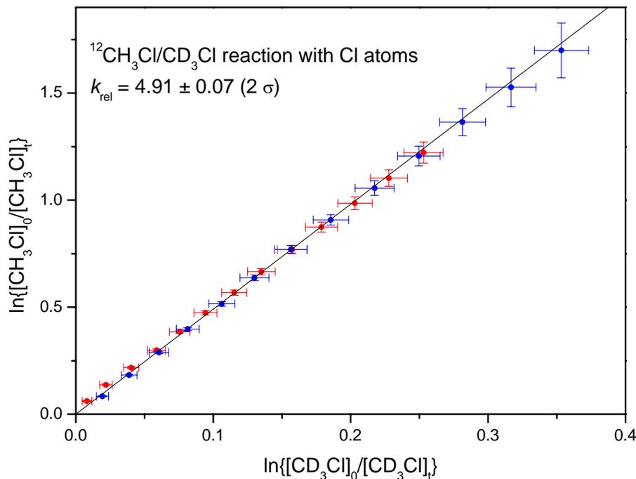
**Fig. 5.** Decays of  $\text{CH}_3\text{Cl}$  and  $\text{CD}_3\text{Cl}$  during reaction with Cl atoms at 1013 mbar and 298 K plotted in the form  $\ln\{[^{12}\text{CH}_3\text{Cl}]_0/[^{12}\text{CH}_3\text{Cl}]_t\}$  vs.  $\ln\{[\text{CD}_3\text{Cl}]_0/[\text{CD}_3\text{Cl}]_t\}$ . 26 data points from 2 experiments (colour coded) were fitted to  $k_{\text{rel}}=4.91\pm 0.07 (2\sigma)$ . Error bars assigned the individual data points correspond to  $1\sigma$  from the spectral analyses.
