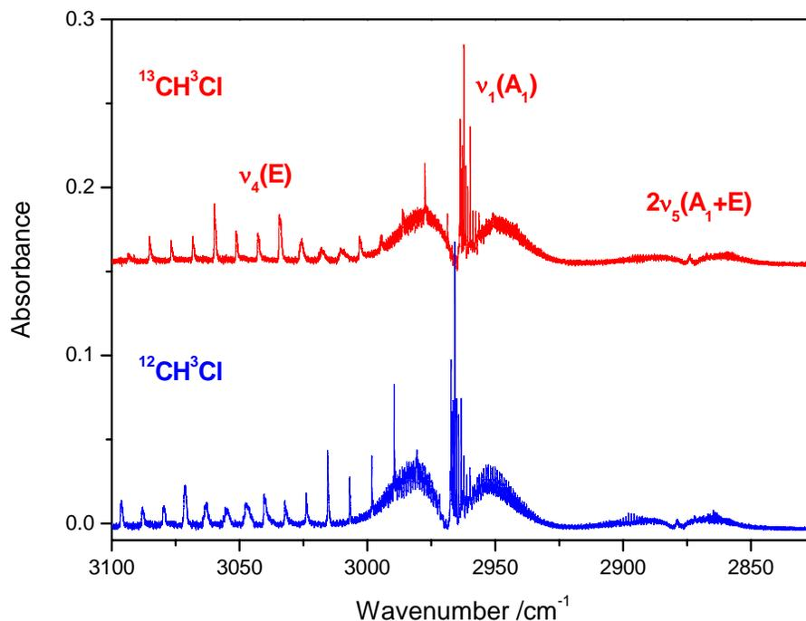
**Fig. 1.** FT-IR spectra in the CH stretching region of a  $\text{CH}_3\text{Cl}$  and  $^{13}\text{CH}_3\text{Cl}$  showing the fundamental  $\nu_1$  parallel band around  $2960\text{ cm}^{-1}$ , the  $\nu_4$  perpendicular band around  $3040\text{ cm}^{-1}$ , as well as the  $2\nu_5$  overtone around  $2875\text{ cm}^{-1}$ . Spectral resolution:  $0.01\text{ cm}^{-1}$ .
