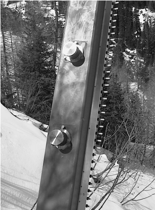
Fig. 1. Detail of flow-height measurements device showing the arrays of electro-mechanical switches spaced 5 cm apart. Cylindrical pressure sensors are visible too.
