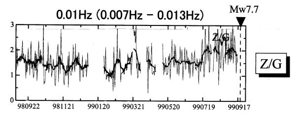
Fig. 2. Temporal evolution of the polarization (Z/G) at a frequency of 0.007 Hz–0.013 Hz during the whole analyzed period. A significant enhancement in the polarization is seen for two months before the quake.
