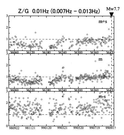
Fig. 3. Effect of changing the threshold on intensity on the temporal evolution of polarization (Z/G) at the same frequency in Fig. 2. The threshold in the top panel is m + s (m: mean and s; standard deviation), m for the middle panel and m - s for the bottom panel.
