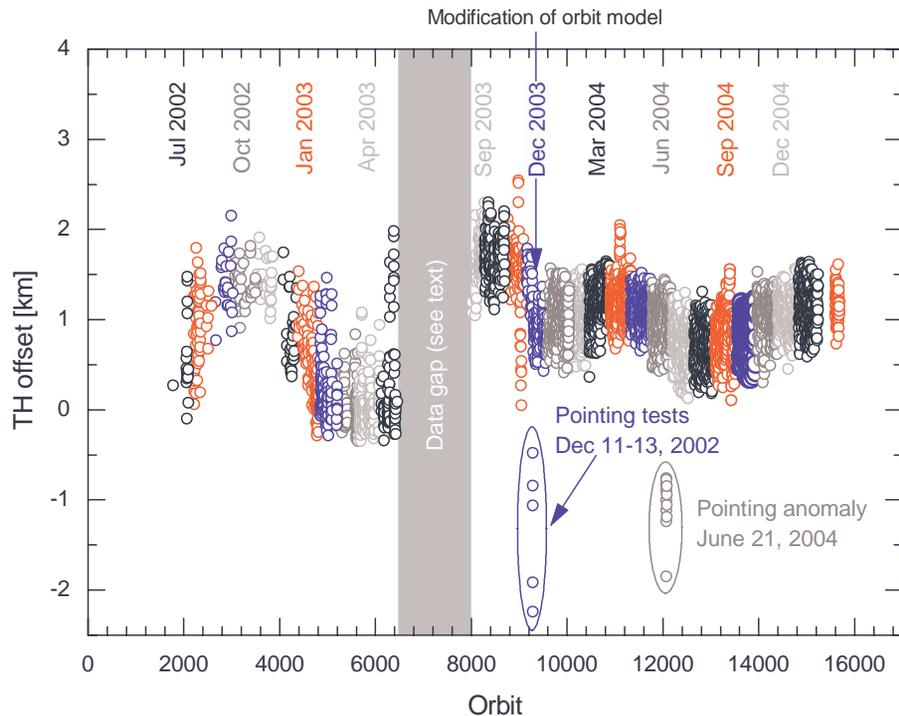
**Fig. 1.** Tangent height (TH) offset retrievals for all available orbits averaged over the tropical limb measurements between  $20^{\circ}$  S and  $20^{\circ}$  N between July 2002 and February 2005. In December 2003 an improvement of the Envisat orbit model took place. Before December 2003 a strong seasonal variation with an amplitude of about 800 m is present. After the update the amplitude is reduced to less than 250 m, but an offset of about 1 km remains.
