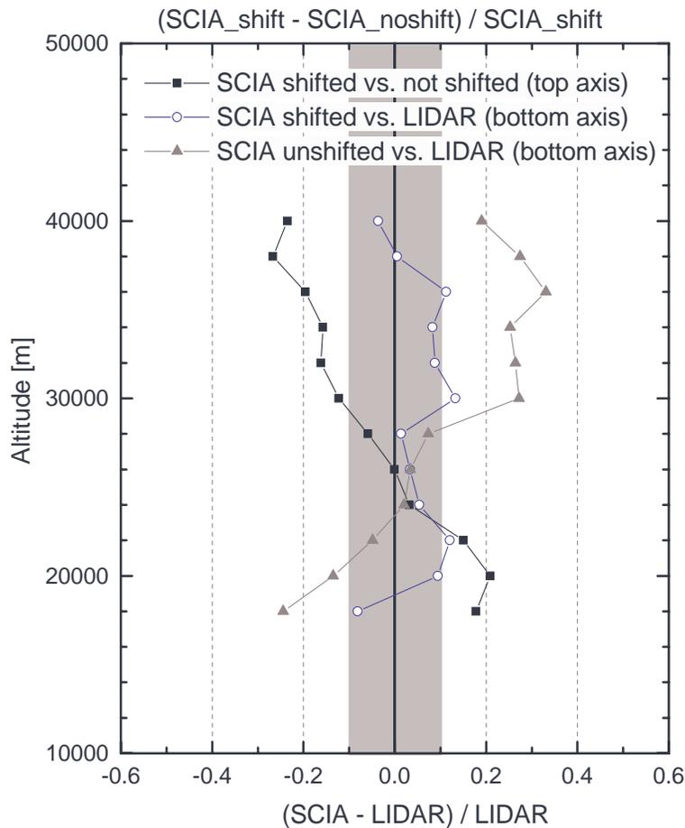
**Fig. 6.** Relative differences between the SCIAMACHY retrievals and the LIDAR measurement and between the pointing corrected and uncorrected SCIAMACHY profiles. The grey shaded area indicates the  $\pm 10\%$  range.
