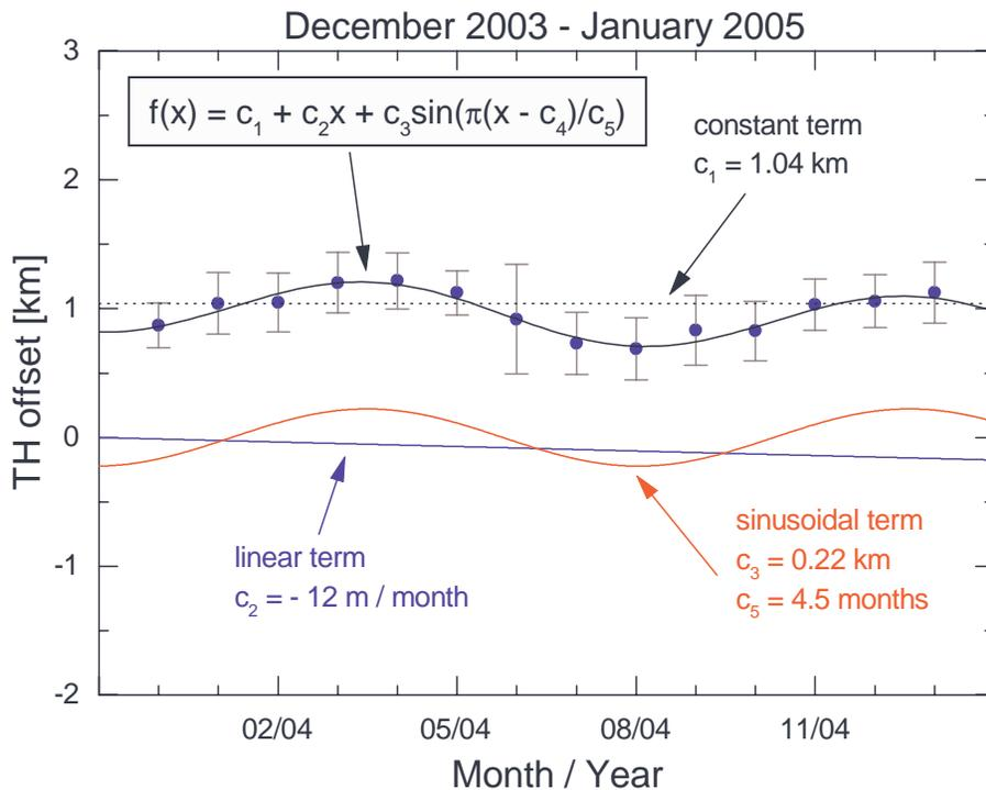
**Fig. 3.** Retrieved and modeled monthly mean TH offsets for the December 2003–January 2005 period. The amplitude of the sinusoidal modulations is reduced to about 1/4 of the value during the July 2002–November 2003 period (Fig. 2). However, a nearly constant offset of approximately 1 km remains.
