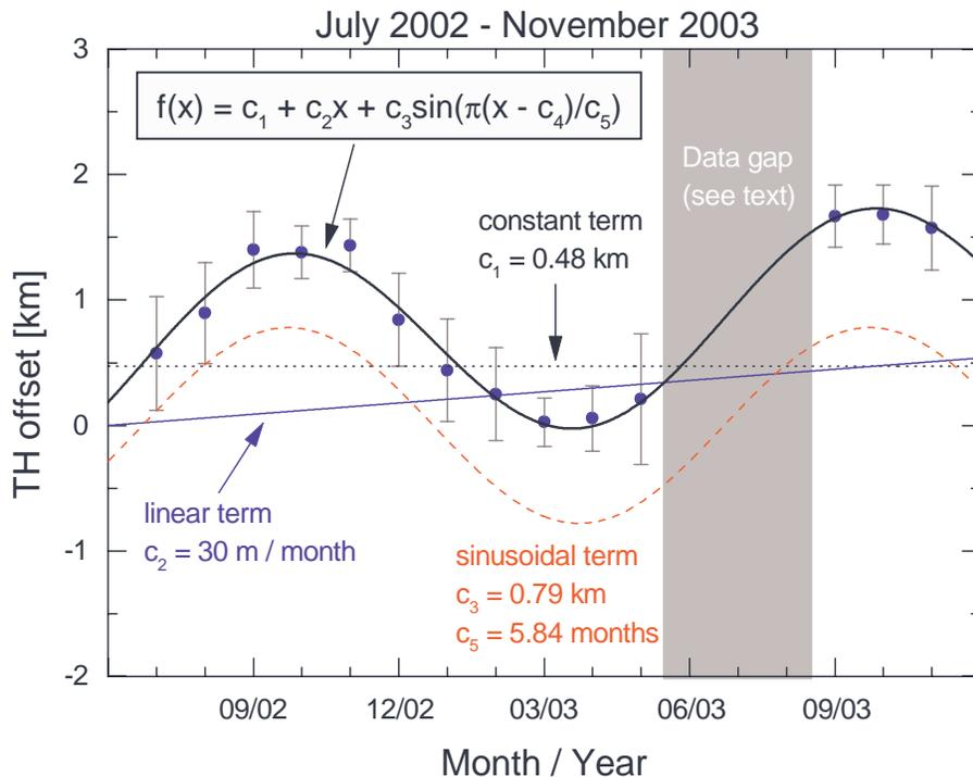
**Fig. 2.** The blue solid circles show the monthly mean TH offsets for the July 2002–November 2003 period. The error bars indicate the standard deviations about the monthly mean values. The TH offset variation was modeled with a superposition of a linear and a sinusoidal function. The amplitude of the sinusoidal function is  $c_3 \approx 800 \text{ m}$ , and its period is  $T = 2 \times c_5 \approx 12 \text{ months}$ .
