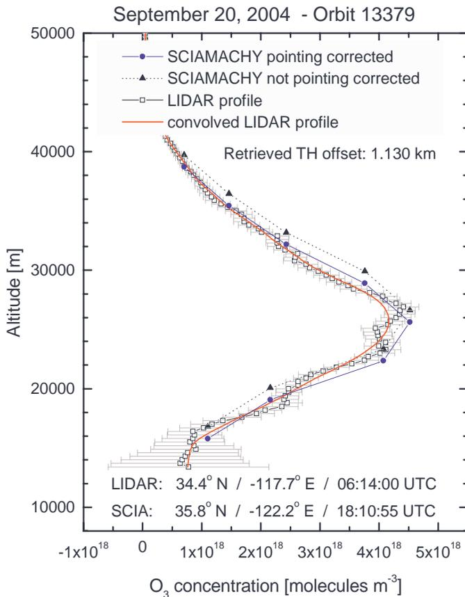
**Fig. 5.** Comparison between SCIAMACHY O<sub>3</sub> profile retrievals with collocated LIDAR measurement on 20 September 2004. SCIAMACHY retrievals were performed with and without the retrieved TH correction of 1.13 km. The red solid line shows the LIDAR profile convolved with the SCIAMACHY averaging kernels. The pointing correction significantly improves the agreement between the LIDAR and SCIAMACHY.
