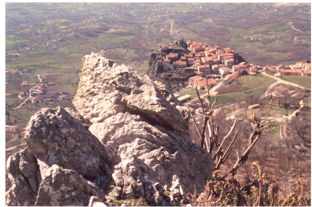
Fig. 9. View of the town of Collianello from the Mt. Marzano southwestern slope. In the foreground, highly fractured limestones, with open or loose joints in the rock mass.
