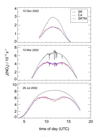
**Fig. 9.** Examples of diurnal variations of  $j(NO_2)$  on the three days of different seasons under clear sky conditions. The external SR data on 10 March 2002 show momentary influence of clouds. SRTM data were scaled by a factor  $h^c = 1.34$ . Data sets start and end at times where the roof of SAPHIR was opened and closed, respectively.
