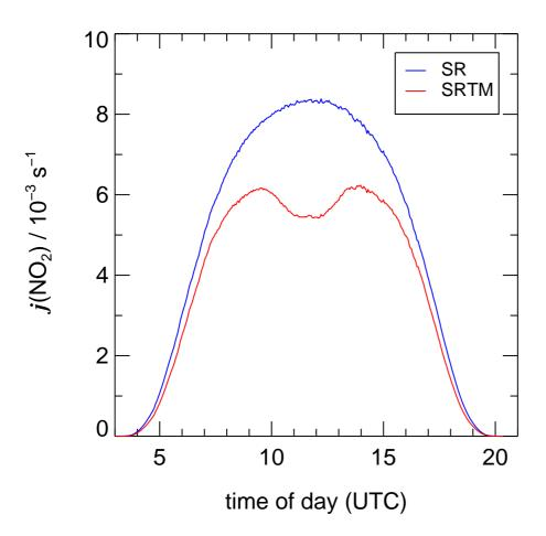
**Fig. 2.** Diurnal variation of  $j(NO_2)$  measured on a clear sky day (28 July 2002) outside the simulation chamber by a spectroradiometer (SR). SRTM predictions for SAPHIR including a preliminary calibration factor of 1.3 (Bohn and Zilken, 2004) are shown for comparison.
