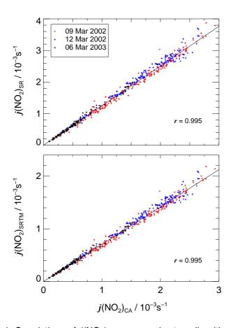
**Fig. 7.** Upper panel: Correlations of  $j(NO_2)_{SR}$  measured externally with a spectroradiometer and  $j(NO_2)_{CA}$  from actinometry inside of SAPHIR on three overcast days. Lower panel: Similar plot with radiometric data modified by SRTM calculations. Linear correlation coefficients r are indicated.
