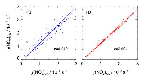
**Fig. 6.** Correlations of  $j(NO_2)_{SR}$  measured externally with a spectroradiometer and inside SAPHIR by actinometry on an overcast day (9 March 2002). Left: photo-stationary calculation (PS), right: time-dependent approach (TD). Linear correlation coefficients r are indicated.
