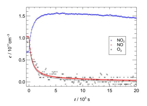
**Fig. 3.** Concentration traces of  $NO_2$ , NO and  $O_3$  after closing the roof of SAPHIR at t=0. Blue, red, and black lines, respectively, show fits from analytical data analysis using NO and  $NO_2$  data.
