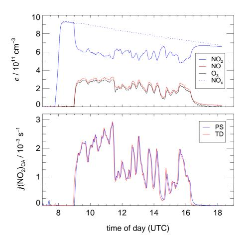
**Fig. 5.** Upper panel: concentration traces of NO<sub>2</sub>, NO and O<sub>3</sub> in an actinometric experiment on 9 March 2002 under overcast conditions. Lower panel: actinometric photolysis frequencies calculated using the photo-stationary (PS) and the time-dependent (TD) approach.
