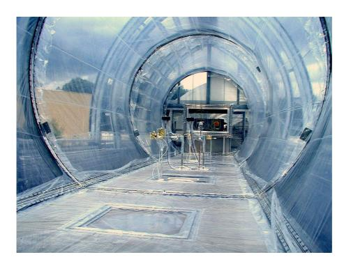
**Fig. 1.** The atmosphere simulation chamber SAPHIR from inside.
