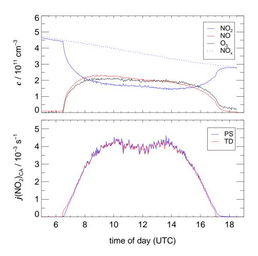
**Fig. 4.** Upper panel: concentration traces of  $NO_2$ , NO and  $O_3$  in an actinometric experiment on 10 March 2002 under clear sky conditions. Lower panel: actinometric photolysis frequencies calculated using the photo-stationary (PS) and the time-dependent (TD) approach.
