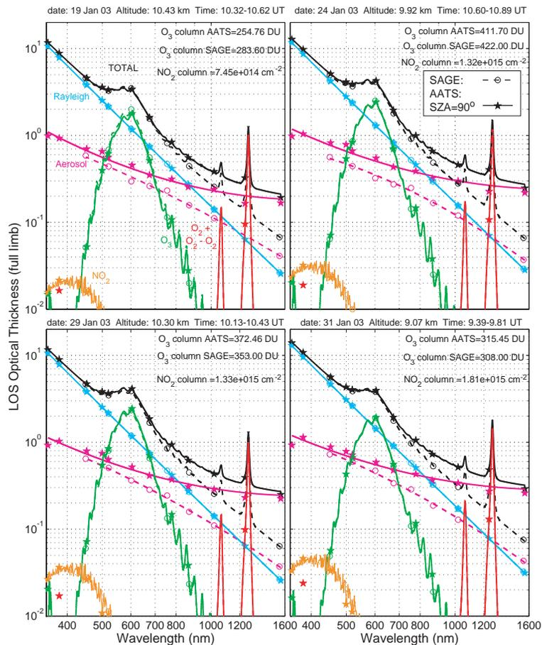
**Fig. 14.** Comparison of AATS and SAGE *LOSOT* (total and components) for 19, 24, 29, and 31 January 2003. AATS values have been converted to apparent  $SZA=90^\circ$ , using the procedure described in Sect. 4 and illustrated in Fig. 12.
