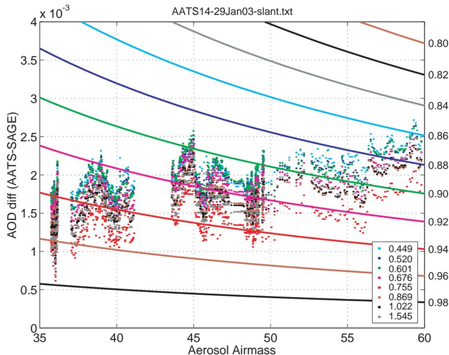
**Fig. A2.** Dependence of AOD difference (AATS minus SAGE) on aerosol airmass, for 29 January 2003. Curves show airmass dependence that would be caused by a window deposit with transmission given by the numbers on the right-hand axis.
