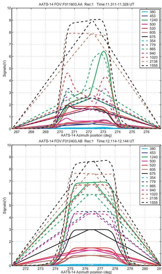
**Fig. A1.** AATS-14 field-of-view (FOV) scans. Top: Made during the DC-8 flight of 16 January 2003, showing the effect of window frost on all channels except 1558 and 2138 nm. Bottom: Made during the DC-8 flight of 24 January 2003, showing the absence of window frost on all channels.
