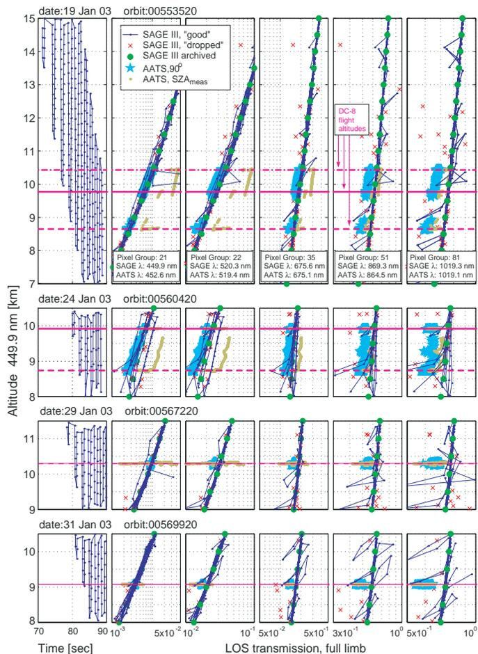
**Fig. 11.** SAGE III vertical profiles of transmission at representative wavelengths for the occultation events near the DC-8 on 19, 24, 29, and 31 January, with near-coincident AATS transmission values at the AATS measurement  $SZA$ ,  $SZA_{meas}$ , and converted to apparent  $SZA=90^\circ$
