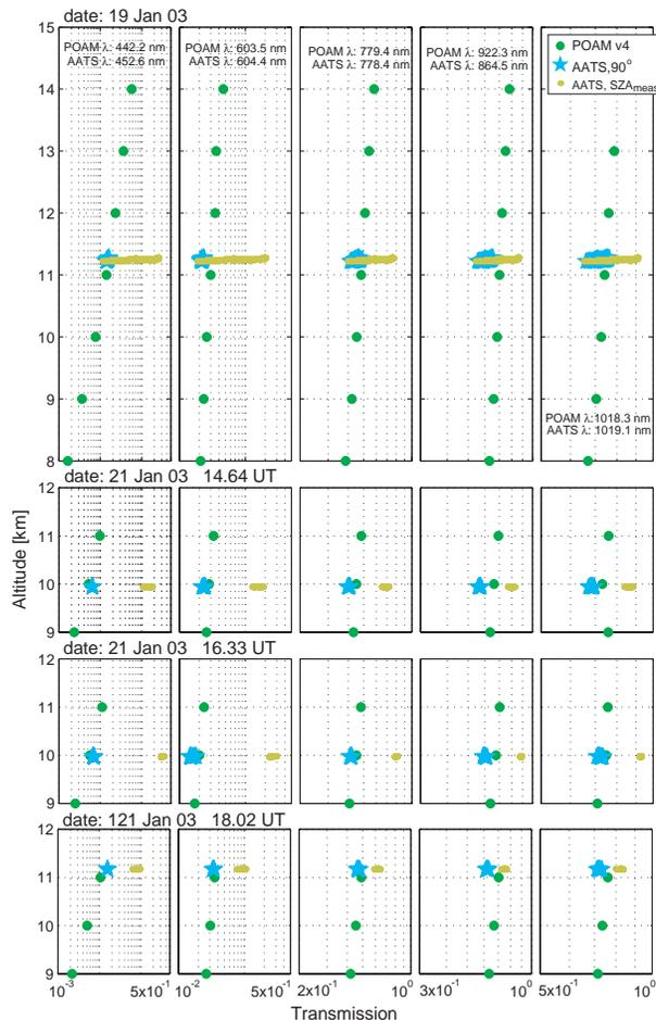
**Fig. 20.** POAM IIIv4 vertical profiles of transmission at representative wavelengths for the occultation events near the DC-8 on 19 and 21 January, with corresponding AATS transmission values (converted from half-limb to full limb) at the AATS measurement  $SZA$ ,  $SZA_{meas}$ , and converted to apparent  $SZA=90^\circ$ .
