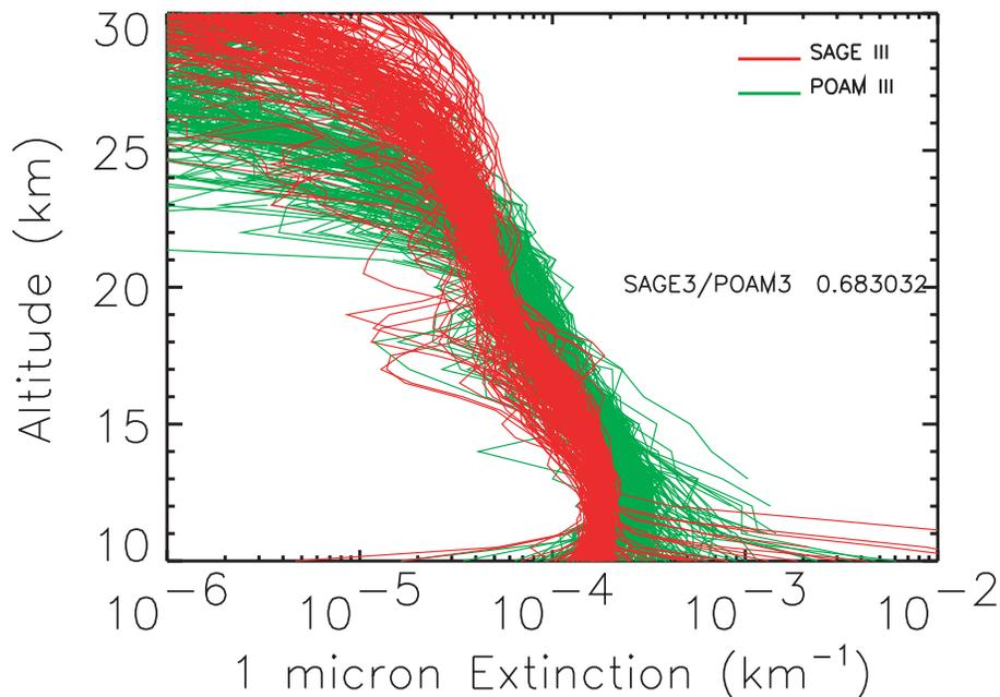
**Fig. 22.** Comparison of POAM IIIv4 and SAGE IIIv3.00 extinction profiles for wavelength 1 micron outside the Arctic vortex and north of 40 N, January 2003. The ratio on the plot is the mean value at 20 km.
