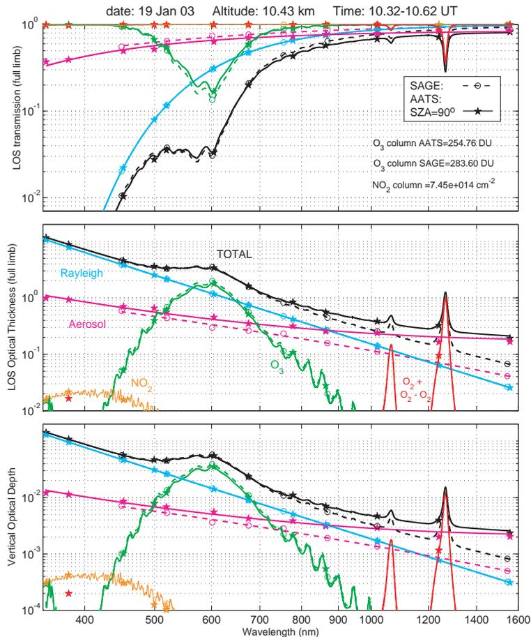
**Fig. 13.** Comparison of SAGE and AATS transmission, *LOSOT*, and *OD*, by components and totals, for 19 January 2003 at 10.43 km. All AATS results for *T* and *LOSOT* have been converted from  $\text{SZA}_{\text{meas}}$  to apparent  $\text{SZA } 90^\circ$ .
