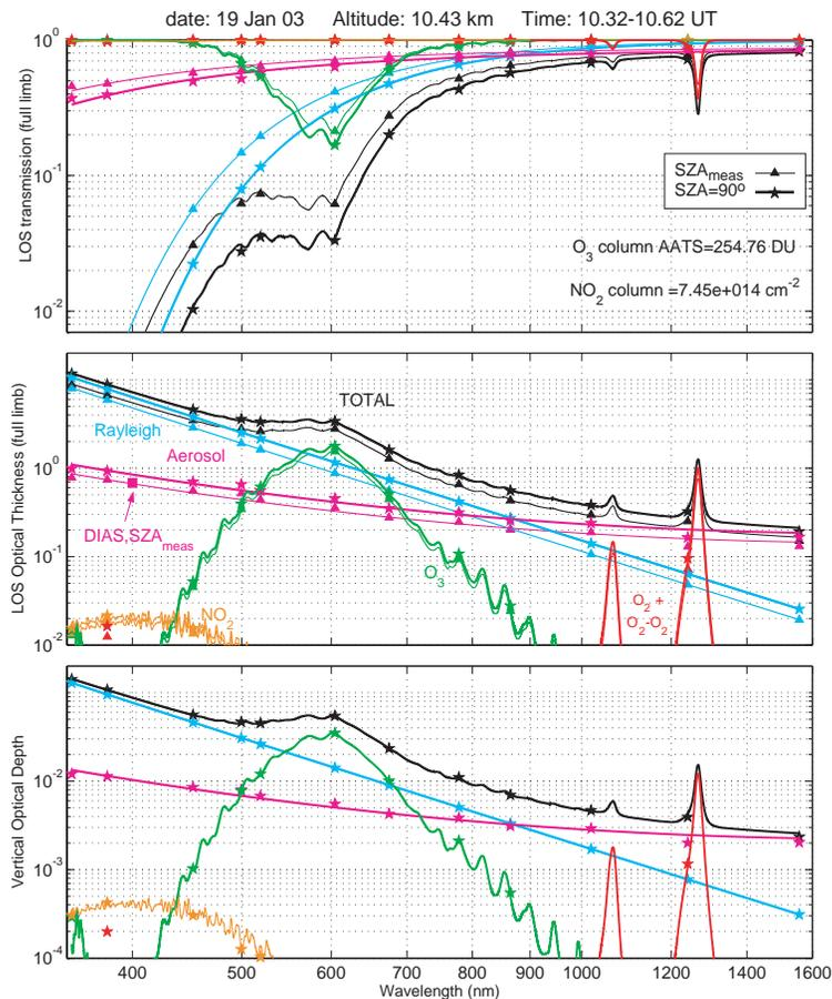
**Fig. 12.** AATS transmission, *LOSOT*, and *OD*, for components and totals, for 19 January 2003 at 10.43 km. **(a)** transmission at  $SZA_{meas}$  and converted to  $90^\circ$ ; **(b)** *LOSOT* at  $SZA_{meas}$  and converted to  $90^\circ$ ; **(c)** *OD*.
