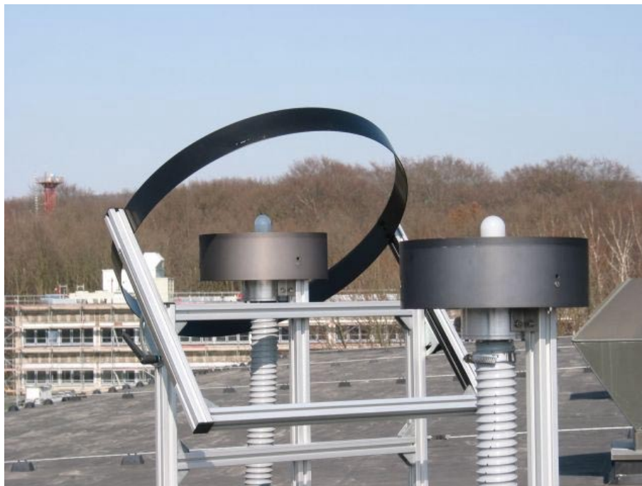
Fig. 2. Actinic flux detector heads of the spectroradiometer with shadow ring obstructing direct sunlight.
