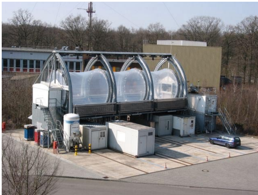
Fig. 1. The atmosphere simulation chamber SAPHIR with opened roof. The photograph was taken from the site of the external spectroradiometer measurements.
