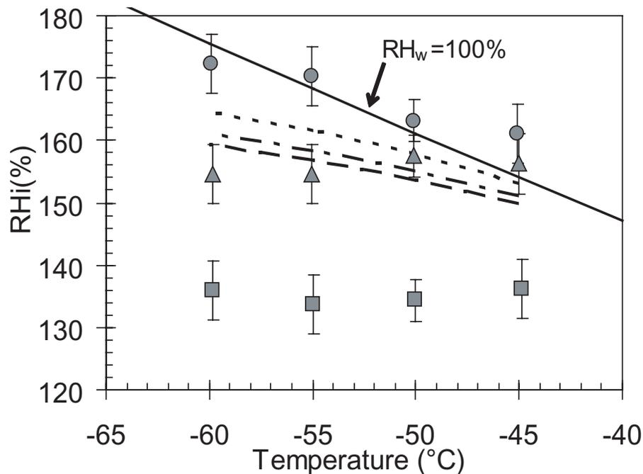
**Fig. 4.** As in Fig. 3, but showing CFDC conditions for the formation of ice on 1% of particles from the sample of resuspended Asian dust. The homogeneous freezing curves are for pure sulfuric acid particles.
