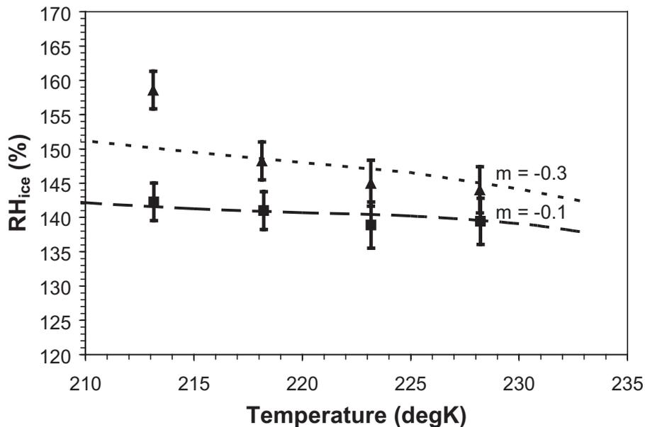
**Fig. 10.** Comparison of classical theory calculations of heterogeneous immersion freezing nucleation with observations for treated iron oxide particles. The data are the points for activation of 1% of particles in the CFDC (95% confidence intervals as error bars). The theoretical calculations are for equivalent 1% activation, as described in the text.
