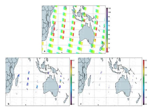
**Fig. 4.** SCIAMACHY SC-AAI on 12 December 2004 over the Indian Ocean, Indonesia and Australia, and the south-western Pacific. **(a)** Sun glint deviation angle of SCIAMACHY ocean pixels. The sun glint deviation angle has a smooth scale, but all pixels satisfying the sun glint condition, i.e. having a sun glint deviation angle lower than 12°, are marked in red. **(b)** SC-AAI without sun glint mask. **(c)** SC-AAI with all ocean pixels with a sun glint deviation angle lower than 12° removed.
