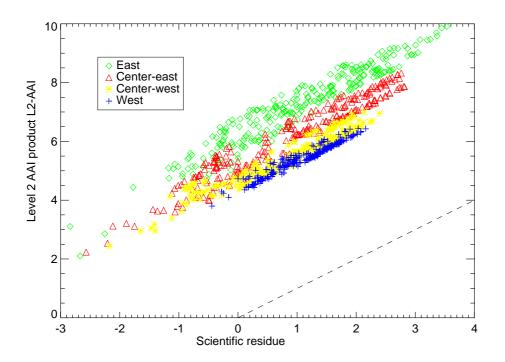
**Fig. 1.** The scientific residue compared to the operational level-2 AAI data for orbit 10 969, states 5–9. The colours refer to pixels with approximately the same viewing geometry. The first four pixels of 30×60 km<sup>2</sup> in a forward swath are called East pixels, the next 4 Centre-east, the next 4 Centre-west and the last 4 West pixels. The dashed line is the one-to-one line.
