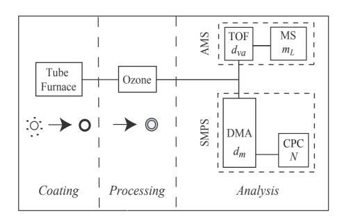
**Fig. 1.** Experimental apparatus for generating, processing, and analyzing coated particles. Key: TOF, time-of-flight; MS, mass spectrometer; DMA, differential mobility analyzer; CPC, condensation particle counter; AMS, aerosol mass spectrometer; SMPS, scanning mobility particle sizer. Symbols  $d_m$ ,  $d_{va}$ ,  $m_L$ , and N are defined in the text.
