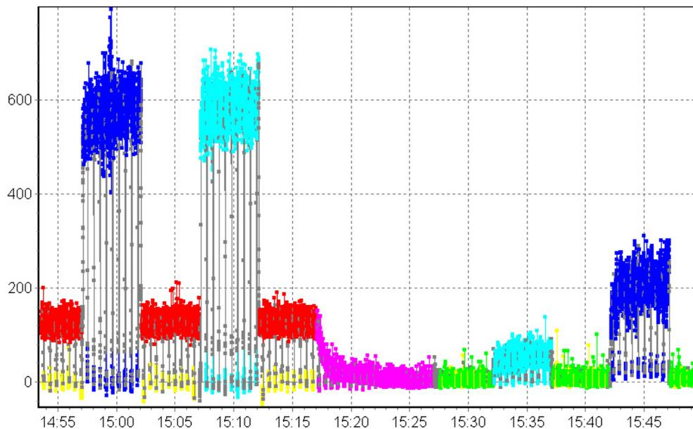
**Fig. 8.** Example for an in-flight calibration cycle (red/green: CLD measure modes ambient air for NO<sub>y</sub> and NO; yellow: CLD zero mode; blue: NO calibration added to ambient in NO<sub>y</sub> and NO modes; turquoise: NO<sub>2</sub> calibration in NO<sub>y</sub> and NO modes; pink: zero air in NO<sub>y</sub> and NO modes).
