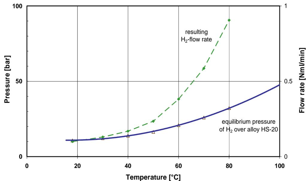
**Fig. 5.** Temperature dependence of the H<sub>2</sub> pressure over the Ti-alloy (triangles) and the corresponding H<sub>2</sub> flow rate (diamonds).
