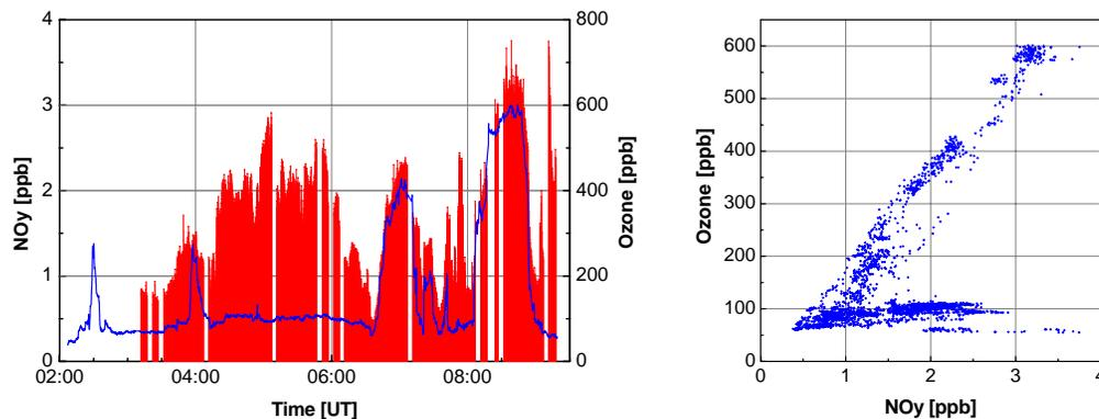
**Fig. 11.** Left: Time series of NO<sub>y</sub> (red bars) and O<sub>3</sub> (blue line) from a MOZAIC flight from Boston to Frankfurt in May 2001. The data gaps are due to calibration and background determinations. Right: Scatter plot of O<sub>3</sub> vs. NO<sub>y</sub>.
