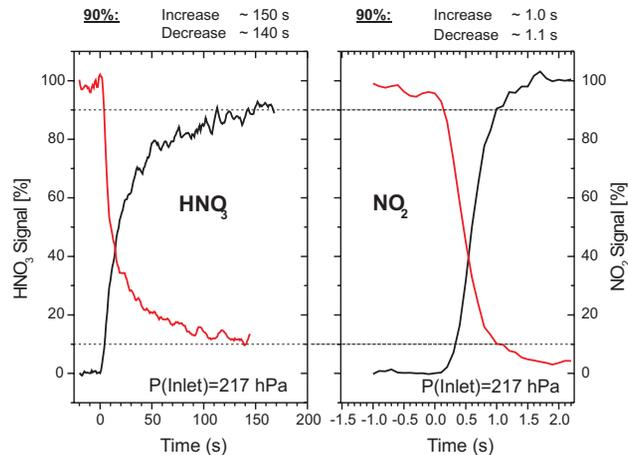
**Fig. 10.** Time response of the gold tube and different inlet line materials (upper panel) and time response of the actual MOZAIC inlet line (80 cm FEP) for NO<sub>2</sub> and HNO<sub>3</sub> (lower panel).
