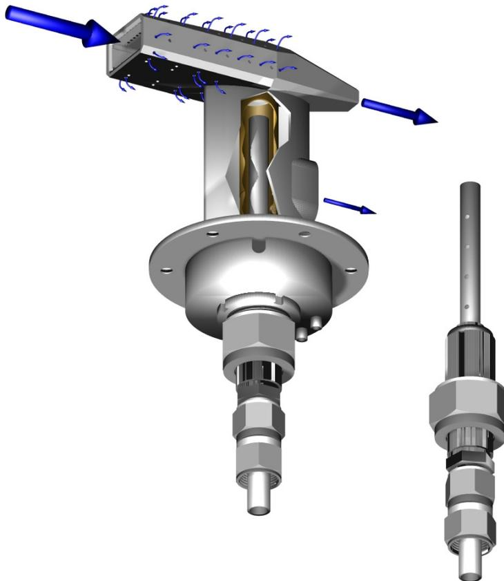
**Fig. 6.** Drawing of the Rosemount probe and the NO<sub>y</sub> inlet line. The arrows indicate the air flow.
