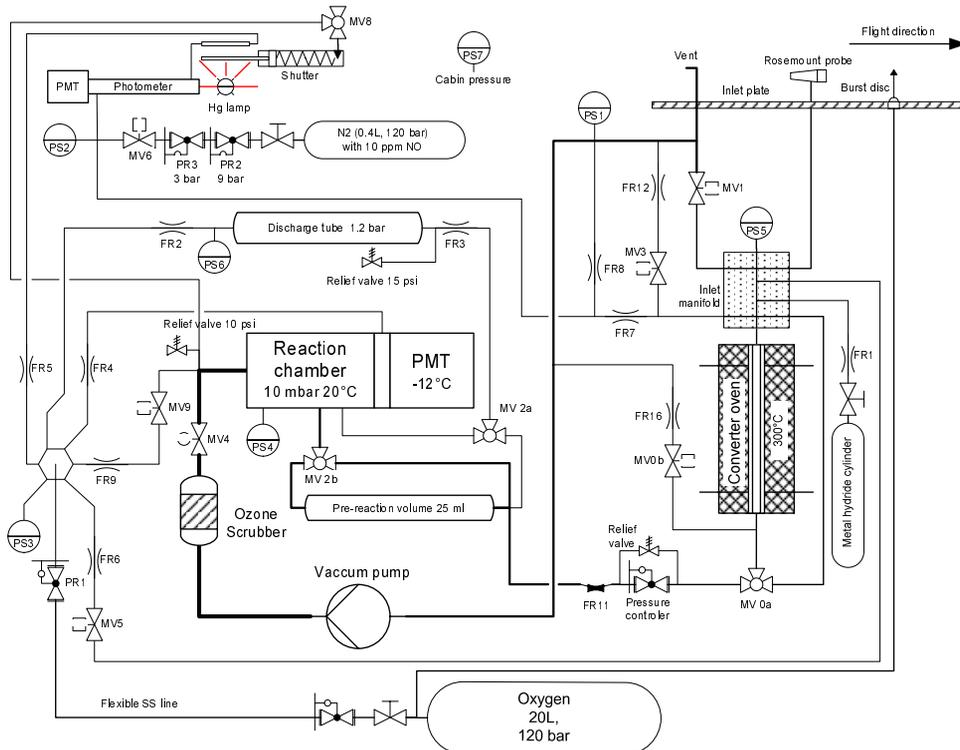
**Fig. 1.** Schematics of the MOZAIC NO<sub>y</sub>-instrument (FR<sub>n</sub>: flow restrictors, i.e., capillaries or critical orifices; PS<sub>n</sub>: pressure sensors; PR: pressure regulators; MV<sub>n</sub>: magnetic valves).
