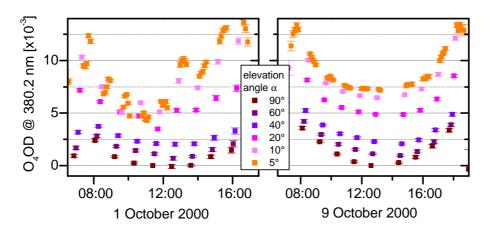
**Fig. 19.** O<sub>4</sub> absorption at different elevation angles in mid-latitudes. Clearly visible is the pattern of increasing O<sub>4</sub> absorption with decreasing elevation angle. The regular pattern shown for a cloud-free day on the right is disturbed only for the lowest elevation angles on a cloudy day (left). The Multi Axis effect is much stronger than the overlaid U-shape pattern which is due to the change in SZA (Leser, 2001; Leser et al., 2003).
