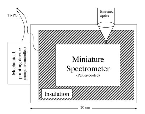
**Fig. 15.** Outline of the Mini-MAX-DOAS instrument. A miniature spectrometer is cooled and temperature stabilized by a 2 stage Peltier cooler. The built-in entrance optics (telescope) provide a narrow field of view (< 0.5°). The unit can be pointed in various directions by computer control.
