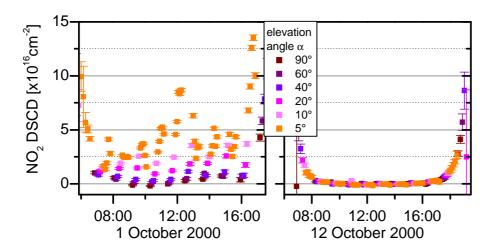
**Fig. 20.** Shown are two examples of NO<sub>2</sub> DSCD's, one for a case with pollution observed in the lower troposphere (left panel, North Sea, 1 October 2000), the right panel shows stratospheric background NO<sub>2</sub> only with no significant differences between the individual elevation angles (Leser, 2001; Leser et al., 2003).
