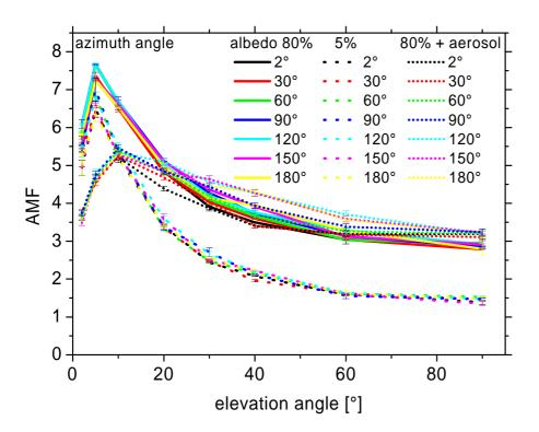
**Fig. 11.** Azimuth-dependence of the AMF for 30° SZA and profile P4 (trace gas layer at 1–2 km altitude). For relative azimuth angles between 2° (looking almost towards the sun) and 180° (looking away from the sun) only a small effect increasing with ground albedo and aerosol load can be seen. Calculations were performed for a ground albedo of 80% and 5% (cf. Fig. 3) in the Rayleigh case (in the troposphere) and for 80% ground albedo in the low aerosol case (cf. Fig. 4).
