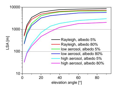
**Fig. 8.** Last scattering altitude (LSA) for pure Rayleigh, low and high aerosol load scenarios (see Fig. 4) and both, 5% and 80% albedo. The LSA is generally below 1km for the lowest elevation angle and above 1km for the highest elevation angles, especially for zenith viewing direction.
