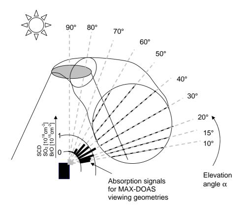
**Fig. 23.** Emission plume monitoring by MAX-DOAS: A volcano as emission source is shown as an example. MAX-DOAS measurements yield spatial information as well as concentration and emission flux data for several trace gases. As an example the viewing directions used by (Bobrowski, 2002; Bobrowski et al., 2003) are sketched and the distribution of the SCD signals of the first scan of Fig. 24 for BrO is included.
