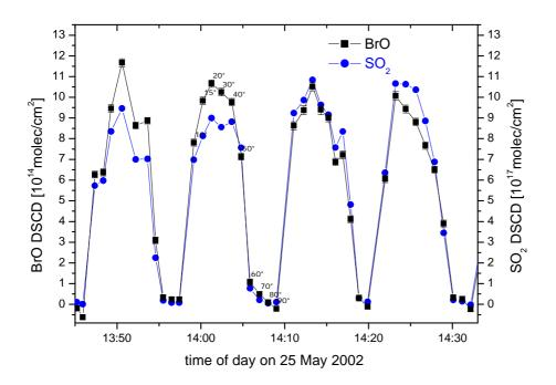
**Fig. 24.** Example of a series of MAX-DOAS scans across a volcanic plume. Volcanic gases like SO<sub>2</sub> and BrO show high DSCD's when the viewing direction crosses the plume, background values are found outside the plume (Bobrowski, 2002; Bobrowski et al., 2003). For the second scan the BrO data points are labelled with the respective MAX-DOAS elevation angle.
