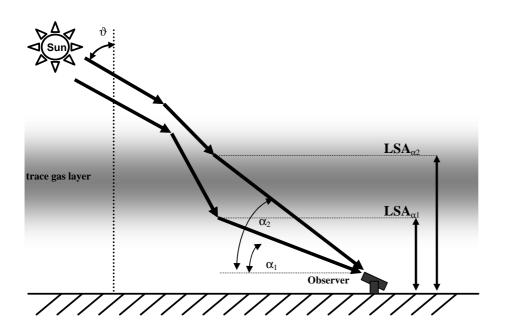
**Fig. 5.** The Last Scattering Altitude LSA: for low elevation angles, the mean free path in the viewing direction is shorter due to higher density and/or aerosol load. This can result in the slant path through absorbing layers at higher altitudes being shorter for lower elevation angles than for higher ones.
