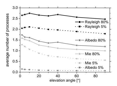
**Fig. 6.** Number of Rayleigh, ground (albedo), and Mie scattering events as a function of elevation angle for the typical rural low aerosol scenario and 5% (dashed lines) and 80% (drawn lines) ground albedo, respectively.
