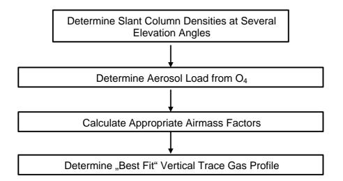
**Fig. 10.** Diagram of a MAX-DOAS evaluation procedure including the determination of the aerosol load from  $O_4$  observations.
