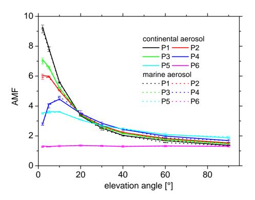
**Fig. 7.** Effect of different aerosol types on the AMF, drawn lines indicate continental background aerosol (same as "low aerosol load" in Fig. 4). Only small differences result from different scattering phase functions.
