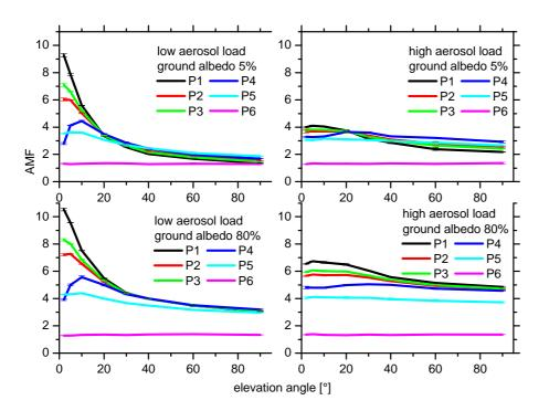
**Fig. 4.** AMF as a function of viewing direction (elevation angle  $\alpha$ ) for P1–P6 for low (left column) and high (right column) aerosol load and for 5% (top panels) and 80% (bottom panels) ground albedo, respectively. Calculations were performed for the same scenario as in Fig. 3, but for typical continental aerosol (left panels: low aerosol load, right panels: high aerosol load, see Fig. 2), differences to marine aerosol are discussed below.
