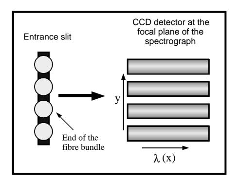
**Fig. 16.** Two dimensional spectrometer: Orientation of the spectra of the measured light from different viewing angles on the CCD array. The dispersion direction is labeled "x", thus for each fibre ending at the entrance slit a complete and separate spectrum is generated on the CCD.
