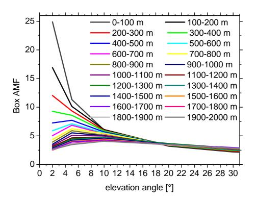
**Fig. 9.** Box AMF for the model layers below 2 km altitude. The sensitivity towards the lowest layers changes strongly for elevation angles below 10°, for elevation angles smaller than 5° the sensitivity already decreases for layers above 400 m altitude.
