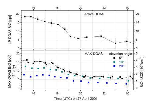
**Fig. 21.** Comparison of active long path DOAS and passive MAX-DOAS BrO measurements at the Hudson Bay for 27 April 2001. From the elevation angle dependence of the  $\Delta$ SCD's a ~1 km BrO layer at the surface can be concluded for e.g. 16:00 h. Using this layer thickness the 5° BrO  $\Delta$ SCD's were converted to mixing ratios for better comparison with the long path DOAS data (Hönninger et al., 2003a).
