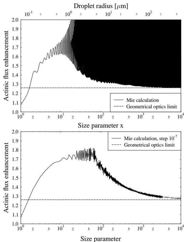
**Fig. 3.** (Top) Mie calculation of the actinic flux enhancement with MIEV and geometrical optics result. The upper x-axis shows the corresponding droplet radius for a wavelength of 400 nm. (Bottom) Same data, but averaged over size parameter bins of width 1.
