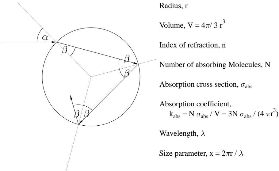
**Fig. 1.** Schematics of a droplet. In the geometrical optics limit, the radiation is traced along individual paths which are considered independent. Refraction is described by Snell's law and reflection follows Fresnel's equations.
