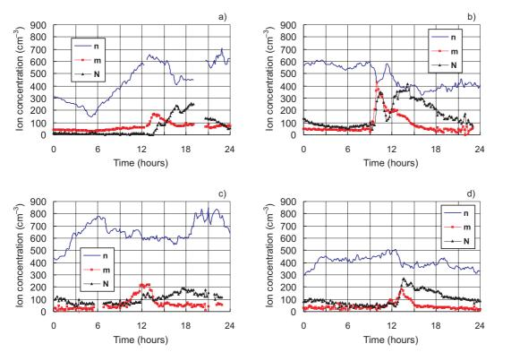
**Fig. 6.** Diurnal variation in the concentration of air ion classes: small ions (n; diameters less than 2.5 nm), charged fine nanometer particles (m; 2.5–8 nm) and coarse nanometer particles (N; 8–ca 20 nm), on 2 April (**a**), 5 April (**b**), 10 April (**c**) and 14 April 1999 (**d**) at Hyytiälä.
