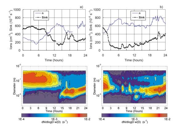
**Fig. 7.** Diurnal variation in the concentration of small ions (*n*), ion sink ( $S_a$ ) and the size distribution of ion sink due to aerosol particles (3–500 nm) on 2 April (**a**; left) and 10 April 1999 (**b**; right) at Hyytiälä.
