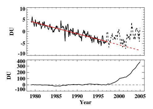
**Fig. 8.** Top: residuals from time-series fit to quasi-global MOD time series with annually-averaged linear trend added back in. Dashed line is the extension of the residuals beyond to fitting time period of 1979–1996. Red line is the linear fit term. Bottom: cumulative sum of residuals from top panel as a function of time.
