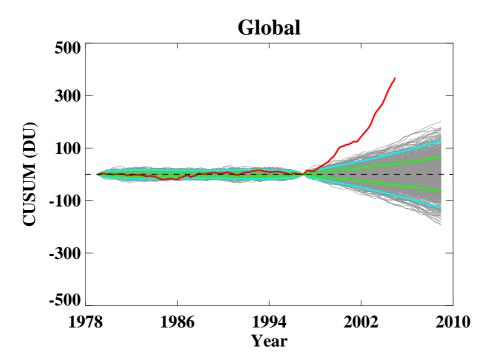
**Fig. 9.** Cumulative sum results without inclusion of instrument uncertainty. The gray region is formed by line plots of 1000 monte-carlo cases used to determine uncertainty. The green thick line is the  $1\sigma$  width of the probability distribution of the 1000 cases as a function of time. The light blue line is the  $2\sigma$  width of the distribution. The red line is the cumulative sum of residuals for the data.
