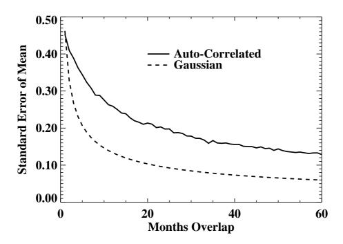
**Fig. 5.** Statistical uncertainty in establishing systematic bias between Nimbus 7 TOMS and Nimbus 7 SBUV as a function of the number of months overlap. Solid line is uncertainty with auto-correlation taken into account. Dashed line is standard error of the mean if data were uncorrelated.
