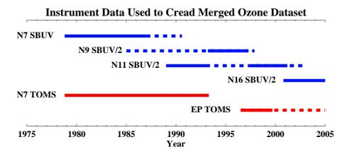
**Fig. 1.** Instruments used to create merged ozone data set. Solid lines indicate time when data was used. Dashed lines indicate time when data was available, but not used for reasons explained in the text.
