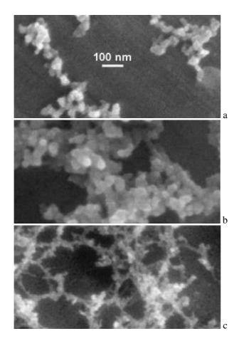
**Fig. 3.** High-resolution SEM images of diesel soot particles in as-prepared samples, **(a)** stage 1 and **(b)** stage 2. **(c)** Residues left behind in stage 2 after sample heating to 600°C. The magnification is the same in all three panels.
