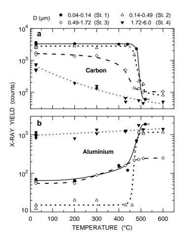
Fig. 8. Comparison of the temperature dependence of X-ray signals measured in the four different size ranges specified at the top, (a) carbon and (b) aluminium.
