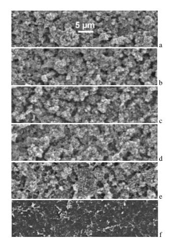
**Fig. 4.** Low-resolution SEM image of stage-1 deposits, **(a)** RT (as-prepared), and after sample heating to different temperatures, **(b)** 200°C, **(c)** 400°C, **(d)** 440°C, **(e)** 480°C, and **(f)** 520°C. The magnification is the same in all six panels.
