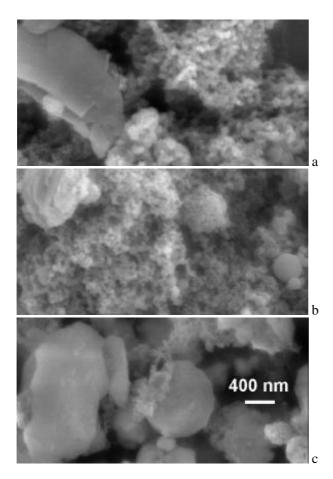
Fig. 2. SEM images showing diesel soot particles (a) in an as-prepared sample (stage 4), (b) after heating to  $300^{\circ}$ C (stage 3) and (c) to  $510^{\circ}$ C (stage 3). The magnification is the same in all three panels.
