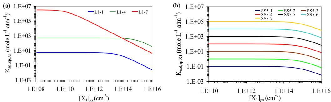
**Fig. 15.** Exemplary numerical calculations for model system Steady-State 6 (SS6), describing equilibrium of a trace gas  $X_1$  undergoing adsorption and surface-bulk transport (non-reactive solvation of a trace gas into a liquid) between the bulk and the gas phases: solubility  $K_{\text{sol,cp},X1}$ , as a function of near-surface gas phase concentration  $[X_1]_{\text{gs}}$  for the parameters defined in model system L1 (a, see Table 2) and model system SS5 (b, see Table 3).
