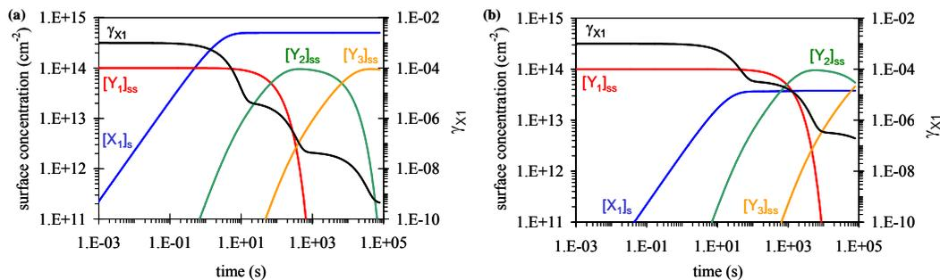
**Fig. 1.** Temporal evolution of particle surface composition and gas uptake coefficient in model system S1 (adsorption and sequential surface layer reactions): scenario S1-1 with  $[X_1]_{\text{gs}} = 2.5 \times 10^{13} \text{ cm}^{-3}$  **(a)** and scenario S1-2 with  $[X_1]_{\text{gs}} = 2.5 \times 10^{11} \text{ cm}^{-3}$  **(b)**.
