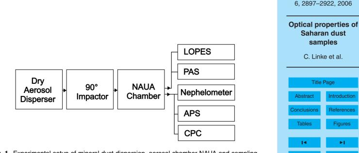
**Fig. 1.** Experimental setup of mineral dust dispersion, aerosol chamber NAUA and sampling. LOPES: Long Path Extinction Spectrometer, PAS: Photo-acoustic Absorption Spectrometer, APS: Aerodynamic Particle Sizer, CPC: Condensation Particle Counter.
