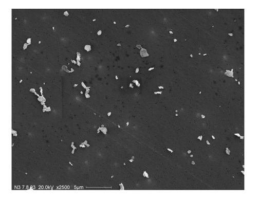
Fig. 6. SEM picture of mineral dust Cairo 3.
