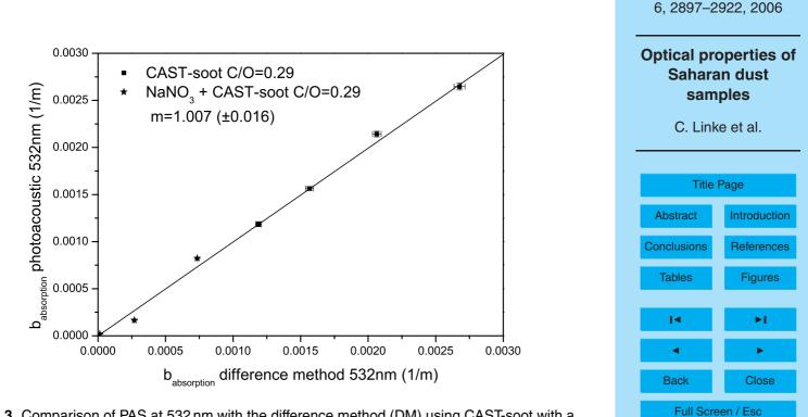
**Fig. 3.** Comparison of PAS at 532 nm with the difference method (DM) using CAST-soot with a C/O ratio of 0.29.
