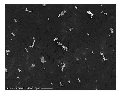
Fig. 5. SEM picture of mineral dust Cairo 2.
