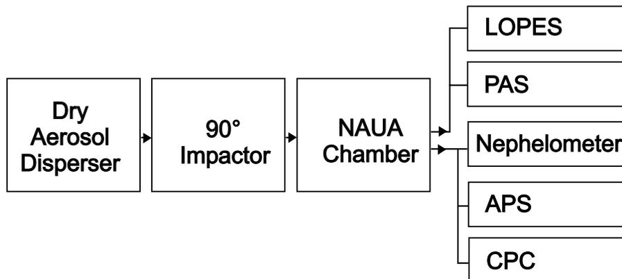
**Fig. 1.** Experimental setup of mineral dust dispersion, aerosol chamber NAUA and sampling. LOPES: Long Path Extinction Spectrometer, PAS: Photo-acoustic Absorption Spectrometer, APS: Aerodynamic Particle Sizer, CPC: Condensation Particle Counter.
