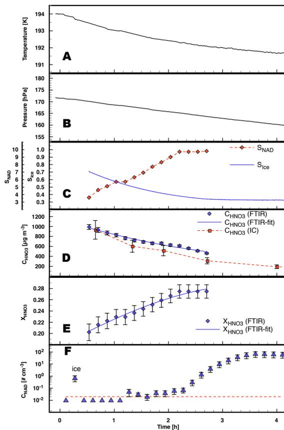
**Fig. 3.** Time series of temperature (panel **A**), pressure (panel **B**), saturation ratios with respect to ice and NAD (panel **C**), aerosol mass (panel **D**) derived from FTIR and ion chromatography (IC), aerosol composition (panel **E**), and ice crystal number concentrations (panel **F**) for experiment E1. For details see Sect. 3.1 of the text.
