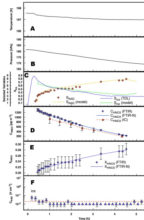
**Fig. 4.** Time series of temperature (panel **A**), pressure (panel **B**), saturation ratios with respect to ice and NAD (panel **C**), aerosol mass (panel **D**) derived from FTIR and ion chromatography (IC), aerosol composition (panel **E**), and ice crystal number concentrations (panel **F**) for experiment E2. For details see Sect. 3.1 of the text.
