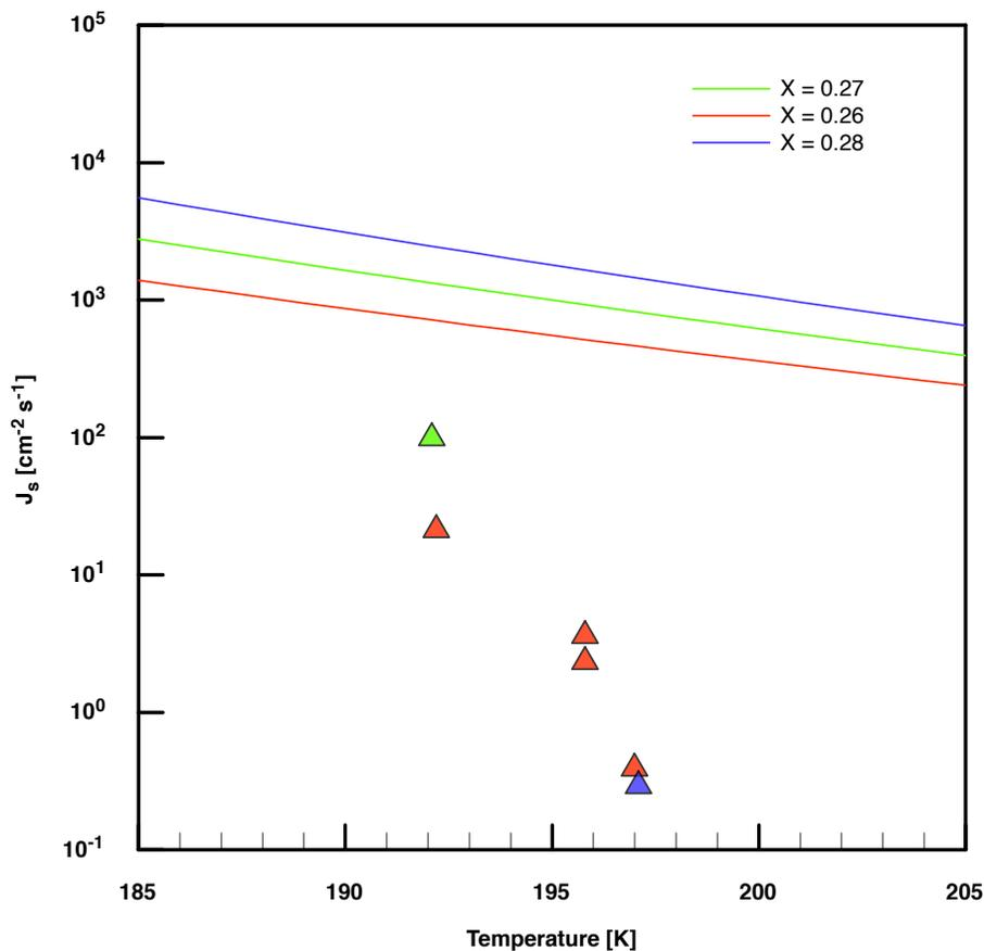
**Fig. 7.** Hypothetical surface nucleation rates calculated from our experimental data (triangles) versus temperature. The parameterisation for  $J_s$  by Tabazadeh et al. (2002) is depicted as a solid lines. The colors represent different molar fractions for nitric acid.
