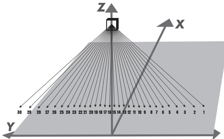
**Fig. 1.** Schematic depiction of the AMSU-A measurements. The satellite is depicted by the square on the  $Z$  axis and orbits along the  $X$  axis. From this platform, AMSU-A performs  $j=1 \dots 30$  sequential step-and-stare measurements at equispaced off-nadir cross-track scan angles  $\beta_j$ , ranging from  $\beta_1=-48.33^\circ$  to  $\beta_{30}=+48.33^\circ$ . Sign convention for quantities on the  $Y$  axis was chosen to preserve a right-handed coordinate system ( $X, Y, Z$ ).
