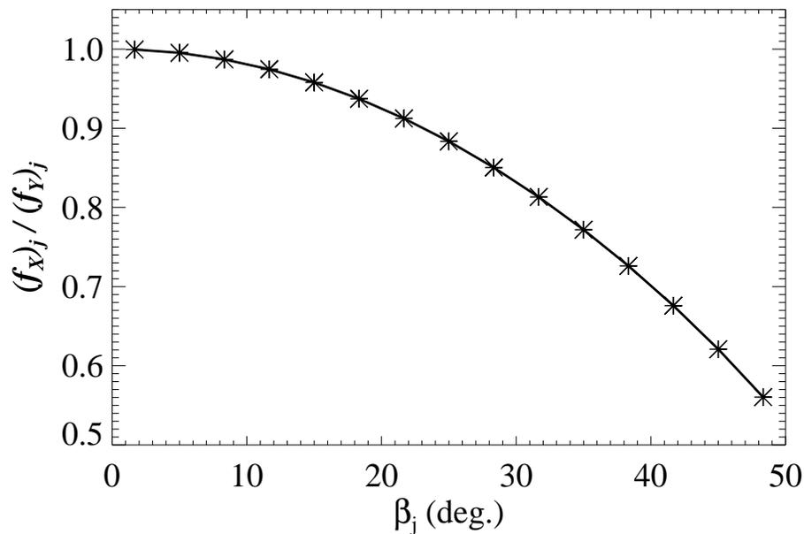
**Fig. 5.** Ratio of along-track to cross-track footprint diameters  $(f_x)_j / (f_y)_j$  versus scan angle  $\beta_j$  based on Eqs. (9) and (10) for NOAA satellite orbit parameters and a nominal Channel 9 measurement altitude of  $Z_C = 18$  km.
