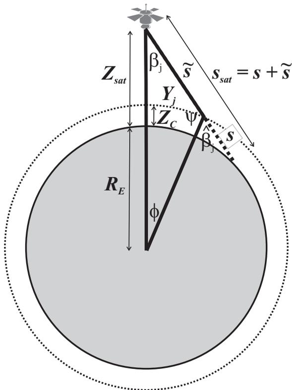
**Fig. 16.** AMSU-A observational geometry. The instrument views the atmosphere at a channel height  $Z_C$  at a scan angle  $\beta_j$ . The line-of-sight distance from this measurement point to the satellite is  $\tilde{s}$  and from the surface to this measurement point is  $s$ .  $Y_j$  is the cross-track swath distance from the subsatellite point to the measurement point. Other symbols are defined elsewhere in the text.
