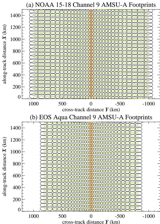
**Fig. 6.** AMSU-A Channel 9 horizontal footprints as a function of along-track and cross-track distances traced out by the AMSU-A scanning pattern from **(a)** NOAA-15 through NOAA-18 satellites and **(b)** EOS Aqua. Orange line shows the satellite ground track. Green curves show the scanning pattern from right-to-left across  $Y$  as the satellite moves along  $X$ .
