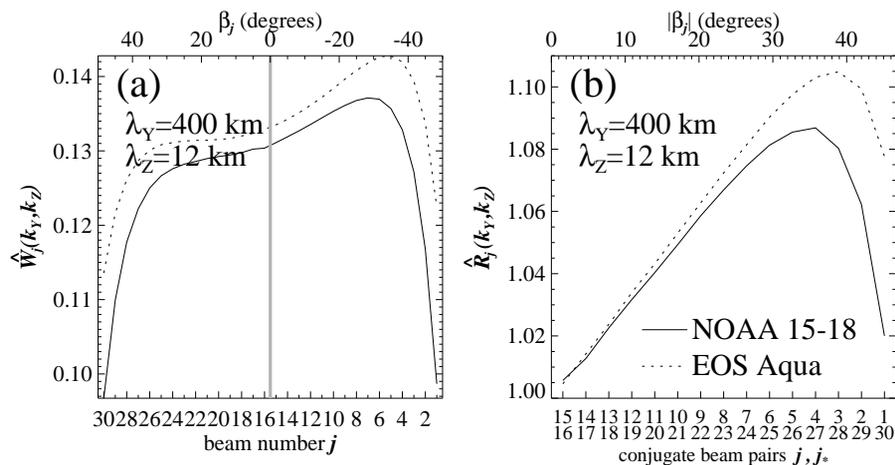
**Fig. 10.** (a) Spectral visibilities  $\hat{W}_j(k_Y, k_Z)$  as a function of beam position  $j$  for  $\lambda_Y=400$  km ( $k_Y>0$ ) and  $\lambda_Z=12$  km ( $k_Z<0$ ) for the AMSU-A on NOAA (solid curve) and EOS Aqua (dotted curve). (b) Ratio  $\hat{R}_{j,j_*}(k_Y, k_Z)$  of the negative scan angle response to the positive scan angle response in (a) for each of the 15 conjugate beam pairs  $j$  and  $j_*$ .
