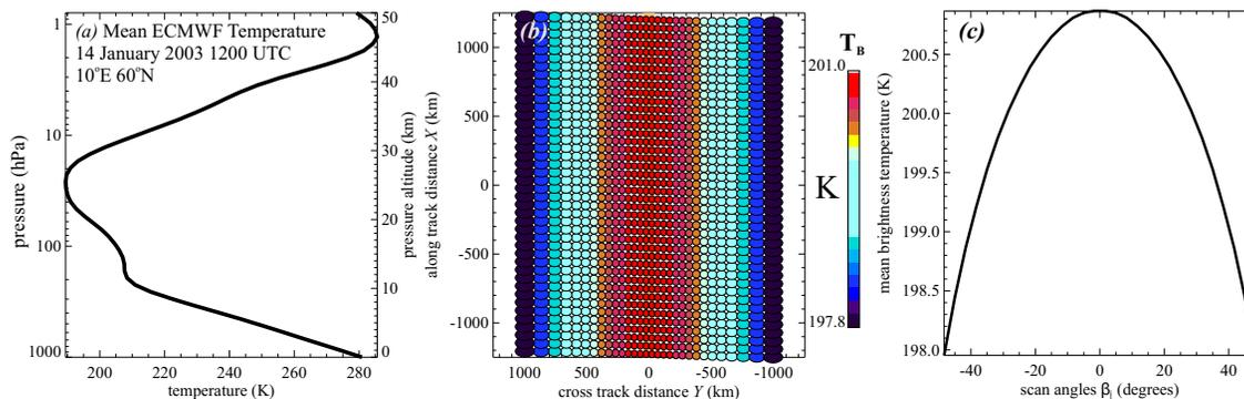
**Fig. 7.** (a) Mean temperature profile from the ECMWF analysis for 14 January 2003 at 12:00 UTC at 10° E, 60° N; (b) model simulation of the AMSU-A Channel 9 brightness temperatures  $T_B(X_j, Y_j)$  obtained from sampling this temperature profile using Eq. (11); (c) mean brightness temperatures from (b) as a function of  $\beta_j$ .
