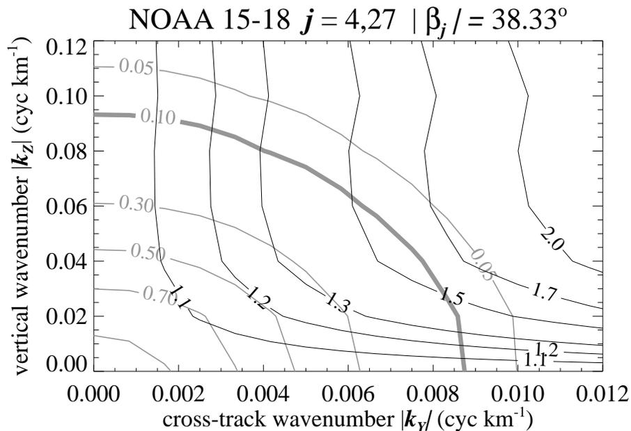
**Fig. 15.** Black contours show the spectral variance visibility ratio  $\hat{R}_{j,j}^2(k_Y, k_Z)$  as a function of cross-track and vertical wavenumber for the NOAA AMSU-A  $j=4, j_*=27$  conjugate beam pairing. Gray lines overlay absolute visibility contours of  $\hat{W}_j(k_Y, k_Z)$  for the  $j=4$  beam.
