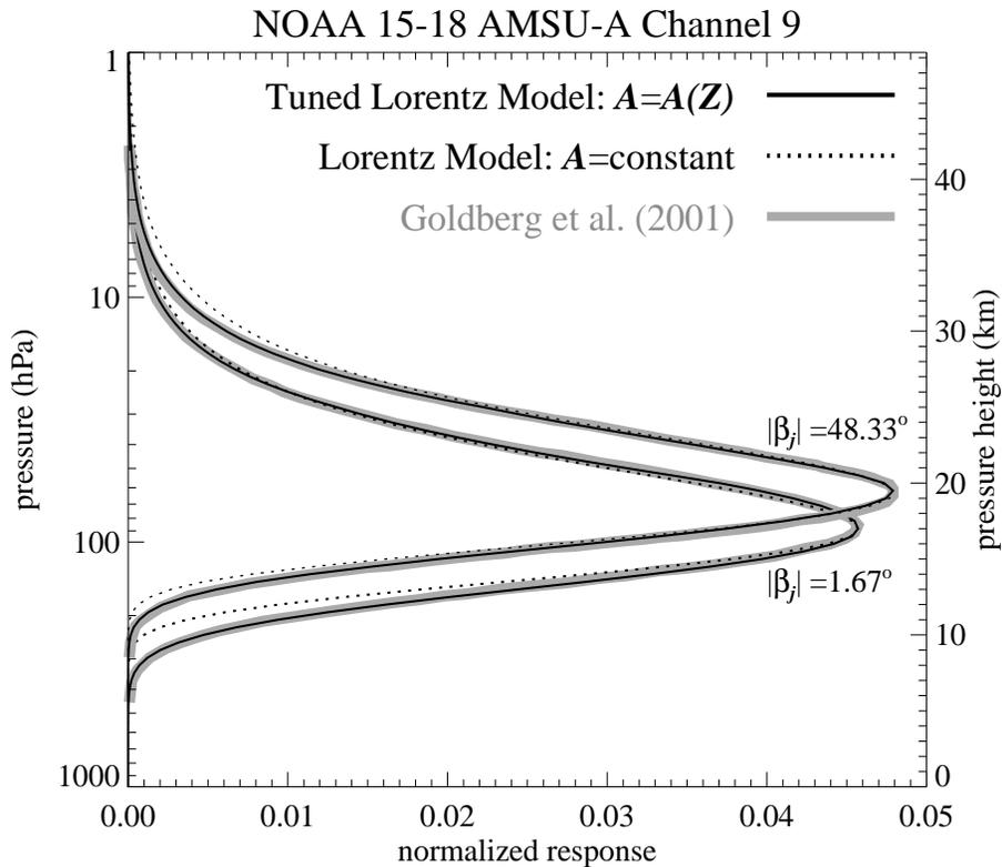
**Fig. 3.** Channel 9 1-D vertical temperature weighting functions  $W_j(Z)$  for the smallest off-nadir angle of  $\beta_j = \pm 1.67^\circ$  and largest off-nadir angle of  $\beta_j = \pm 48.33^\circ$ , derived from our simple Lorentz model (constant  $A$ ; dotted curve) and tuned Lorentz model (height-varying  $A$ , solid curve). Gray curves show results using complete models of radiative transfer and instrument specifics, taken from Goldberg et al. (2001).
