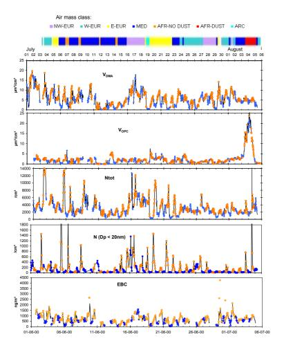
**Fig. 5.** Time series of various aerosol parameters during the MTC campaign. Yellow dots: day time data; blue dots: night time data. Time axis indicates local time (UTC+2). The colored bar on top indicates the air mass category as a function of time.
