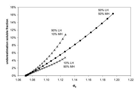
**Fig. 3.** Calculated error on the soluble fraction (Eq. 2) when a bimodal GF distribution (each mode with  $\sigma$ =1.07) is treated as a single lognormal mode, as function of the  $\sigma_g$  of the overall GF distribution.
