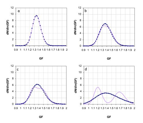
**Fig. 2.** Analytically generated GF distributions from perfectly internally mixed **(a)** to gradually increasing externally mixed **(b)**, **(c)**, **(d)**, by separating the GF into two modes with increasing distance (full line, violet). The dotted blue line represents a hypothetical single mode GF distribution based on average GF and width of the bimodal distributions (see Eq. 1 and text). Case b illustrates the difficulty to recognize two merged modes.
