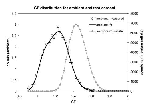
**Fig. 1.** Hygroscopicity measurement with T-DMA of ambient and test aerosol (ammonium sulfate), together with lognormal fit (full line). The distribution width of the test aerosol is the minimum width of a perfectly internally mixed aerosol.
