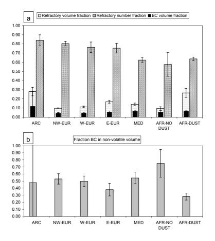
**Fig. 11.** Refractory number and volume fraction, and BC volume fraction for the different episodes **(a)**; contribution of BC to the refractory fraction **(b)**.
