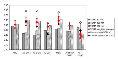
**Fig. 10.** Soluble fraction calculated from the *GF* measurements for 50, 100, and 200 nm particles (vertical bars), and volume-weighted average for the average size distribution (red dots). White diamonds: soluble fraction calculated from chemical composition, using ions + water soluble organic matter (see text). Black diamonds: idem, excluding water soluble organic matter.
