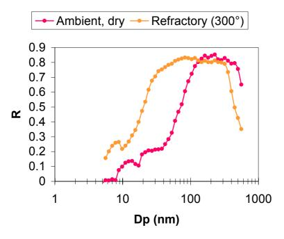
**Fig. 7.** Correlation coefficient between black carbon concentration and aerosol number within a narrow diameter bin for ambient temperature (red) and refractory aerosol (orange).
