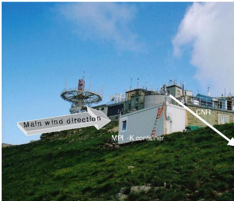
**Fig. 2.** A measuring container housing the CIMS instrument was set up upwind from the CNR station with respect to the main wind direction (prevailing winds blow from SW) as indicated. A blow-up of the sampling line is shown in the right lower corner. In this way ambient air was sampled approximately 4.5 m above the ground and about 1 m above and in front of the container. The inlet pointed outwards towards the edge of the southern mountainside of Monte Cimone, i.e. in the main wind direction.
