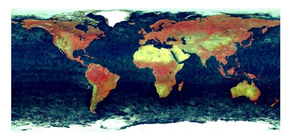
**Fig. 1.** Earth surface as seen by SCIAMACHY PMD 2, 3, and 4, as blue, green and red, respectively. The Earth surface was gridded to  $0.25^{\circ} \times 0.25^{\circ}$  cells, with each grid-cell filled with the darkest PMD 2 (blue) intensity between November 2002 and October 2003. Some cloud-structures are still present. The image shows a reddened Earth as the PMD 4 is in the near infrared and not red.
