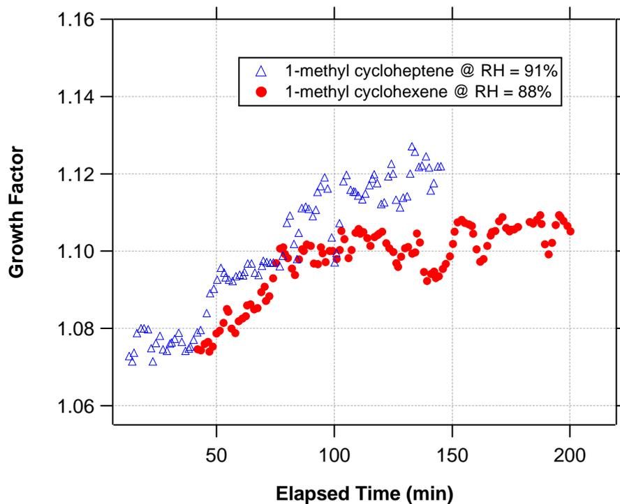
**Fig. 5.** The growth factor of nucleated cycloalkene ozonolysis SOA increases with time early in experiment, consistent with further oxidation of organic products into more polar and more hydrophilic species.
