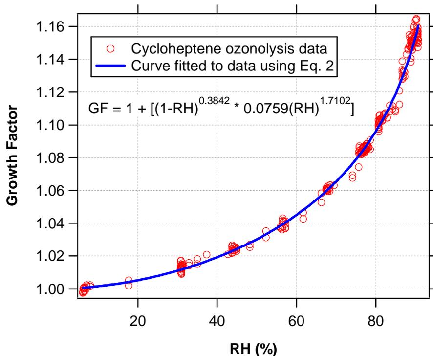
**Fig. 6.** Hygroscopic growth factor as a function of  $RH$  for nucleated SOA formed by ozonolysis of 170 ppb of cycloheptene. The growth curve is smooth, and no deliquescence or efflorescence is observed. The fitted curve is the empirical three-parameter fit of the form of Eq. (2).
