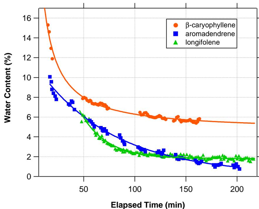
**Fig. 8.** The liquid water content of nucleated sesquiterpene photooxidation SOA decreases with time during the experiment, suggesting that the SOA is becoming less hygroscopic. This behavior is consistent with the continued formation of less hygroscopic oligomeric species. The data shown are from 180-nm classified particles.
