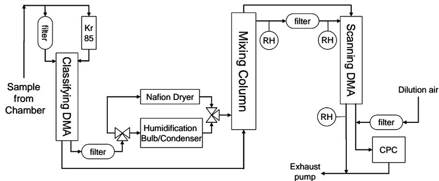
Fig. 1. Schematic of the HTDMA system used.
