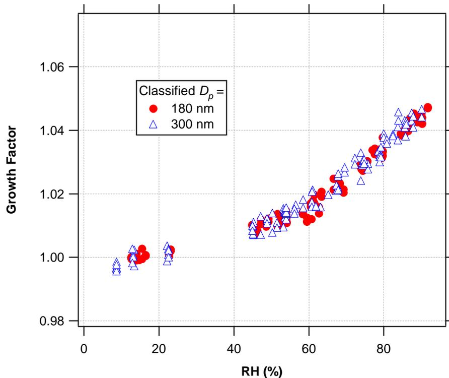
**Fig. 9.** Different classified diameters of pure  $\beta$ -caryophyllene photooxidation SOA exhibit similar hygroscopic growth factors, suggesting that the aerosol composition is independent of particle size.
