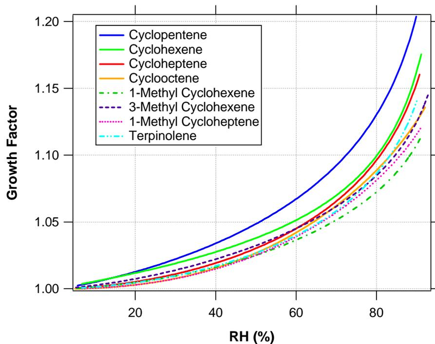
**Fig. 7.** Fitted curves of hygroscopic growth factors as a function of  $RH$  for nucleated SOA formed by ozonolysis of various cycloalkenes. Fitting parameters used to generate the curves are given in Table 3. In general, pure cycloalkene ozonolysis SOA is slightly hygroscopic, with GF between 1.09–1.16 at 85%  $RH$ .
