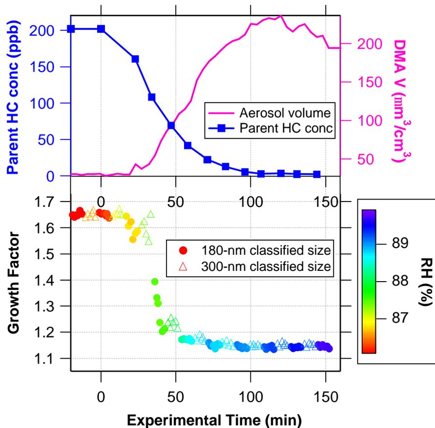
**Fig. 3.** Aerosol hygroscopic growth factor decreases as the precursor cycloalkene is consumed and the gas-to-particle partitioning of organic products occurs onto  $(\text{NH}_4)_2\text{SO}_4$  seed. The data points shown are from a 202 ppb 1-methyl cyclohexene + ozone experiment.
