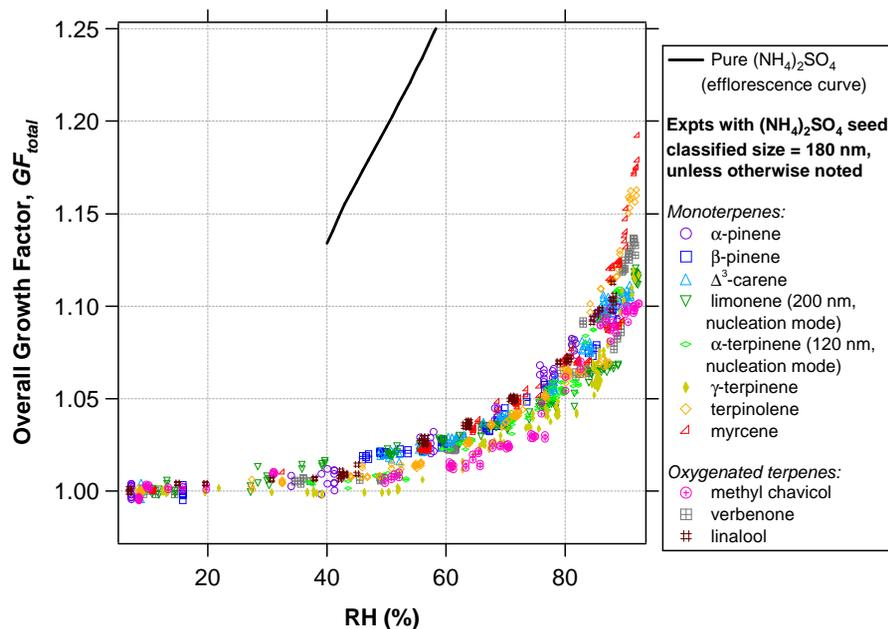
**Fig. 13.** Raw hygroscopic growth factors of SOA from monoterpene and oxygenated terpene photooxidation (with  $(\text{NH}_4)_2\text{SO}_4$  seed). Reported data are from 180-nm classified diameter, unless otherwise noted. All the growth factors from various terpene precursors are contained within a relatively narrow envelope between 1.06–1.11 at 85% RH.
