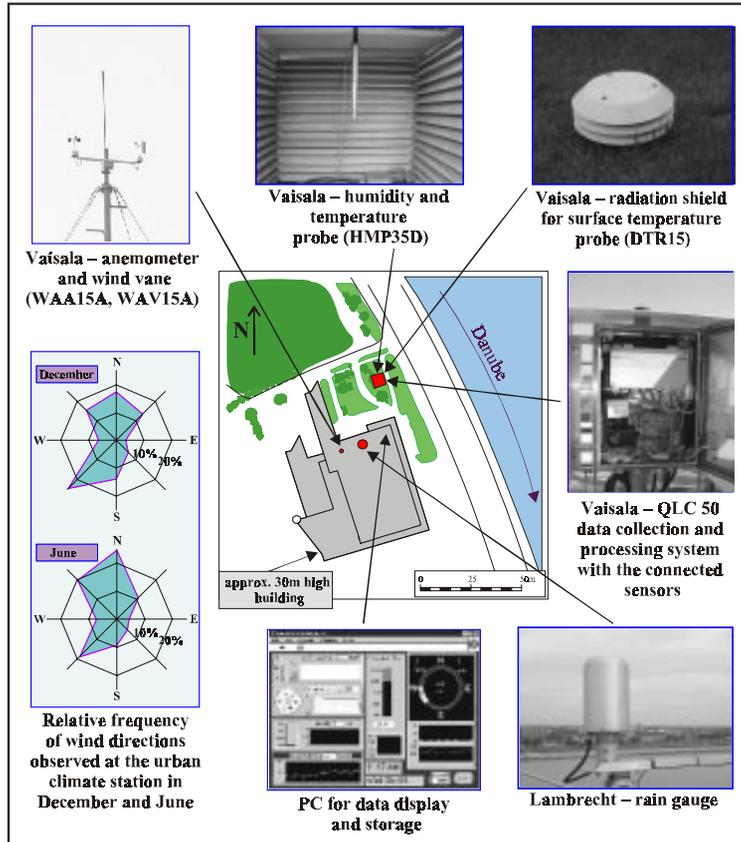
**Fig. 2.** Urban climate station at the Eötvös Loránd University (Budapest, Hungary) installed and maintained with the co-operation of the Hungarian Meteorological Service.
